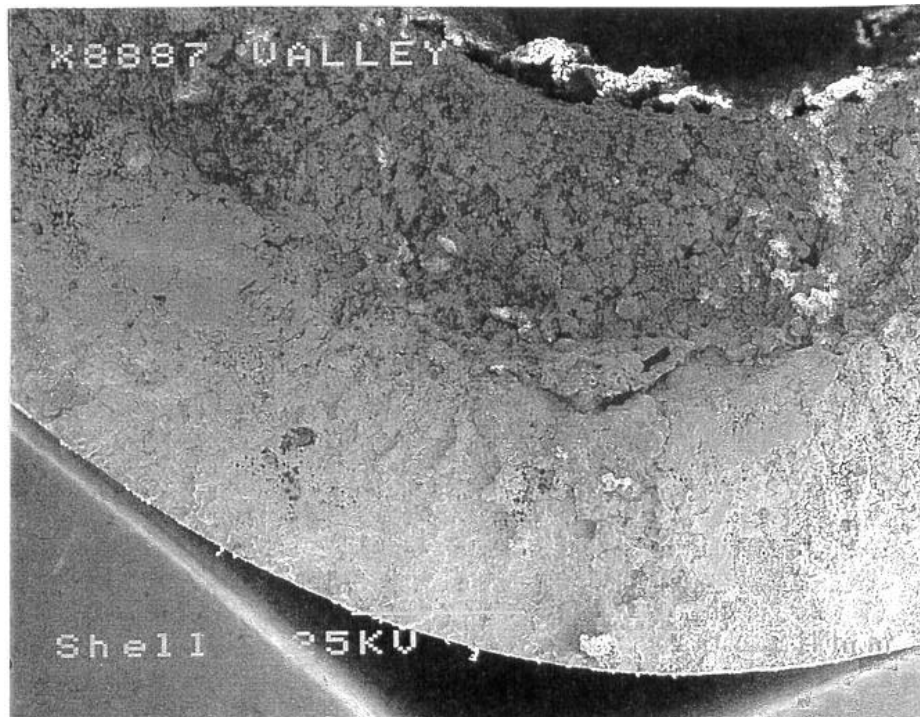
Figure E-18: 25X magnification fractograph displaying a portion of the fracture face of the dowel pin which broke in the service of the 36" Clow check valve.
