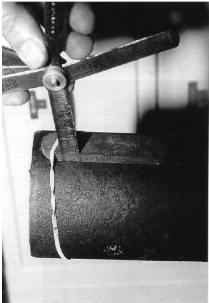
Figure E-13: Photograph shows the metal key intended to help mechanically connect the drive shaft to the valve disk.
