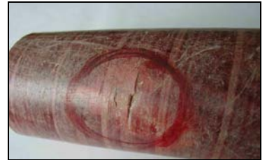
Fiberglass piping is cracked
