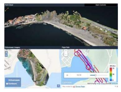
application is built on several open access software packages. It uses Potree, a WebGL based point cloud viewer for very large datasets, to present 3D imagery and serves imagery data from a local GeoServer and UAV flight paths from a cloud-based CartoDB mapping system. Stief indicated that the presented layout, and others like it, can be utilized for research, outreach/ education and commercial purposes. (Presented by Johnston).
