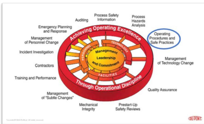
Figure 39. Where Shift Communication Falls on DuPont's PSM Wheel [54, p. 2]. Source: DuPont, with annotations by CSB.
