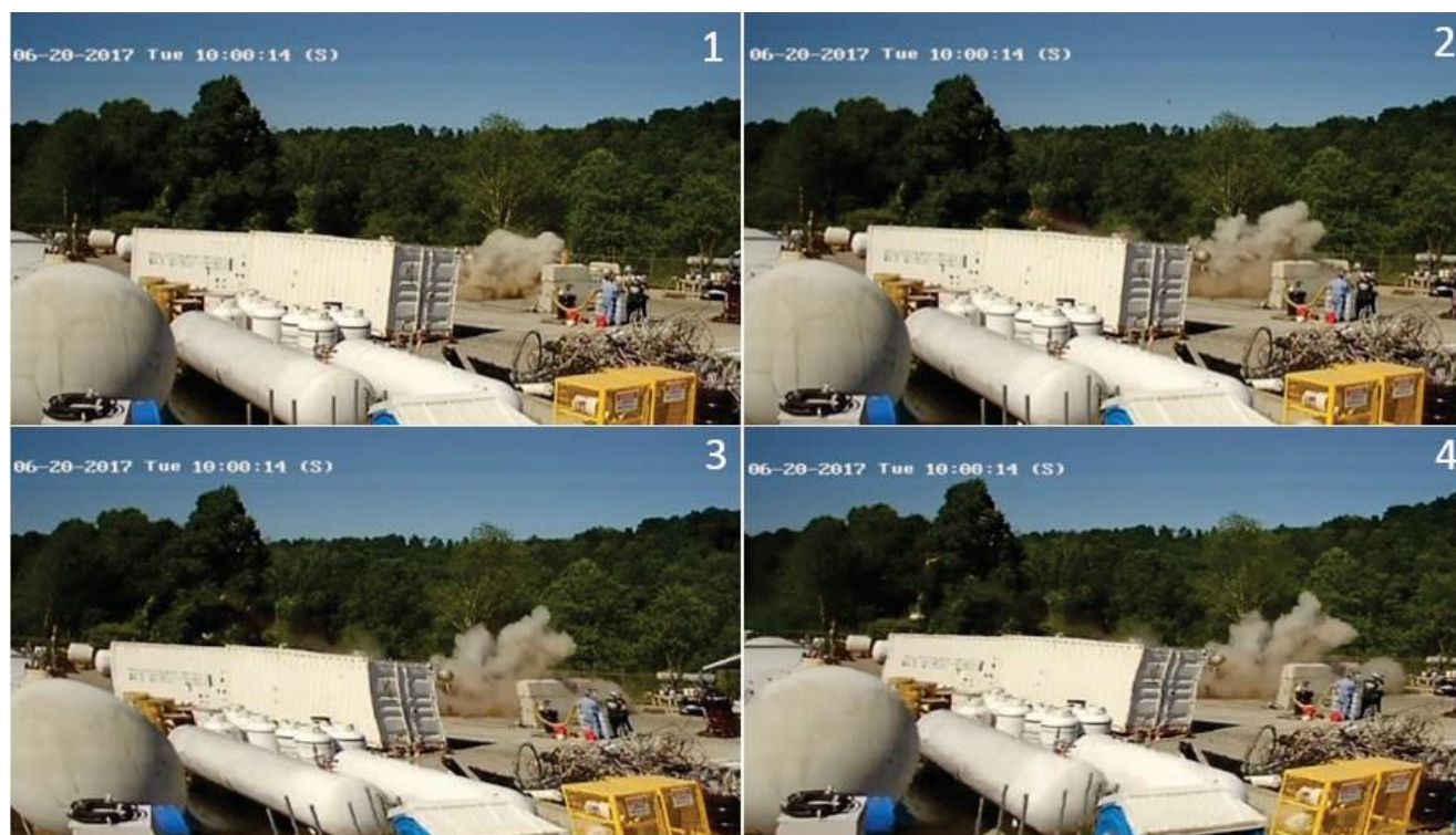
Figure 15. Surveillance Video Capturing June 20, 2017, Explosion. These still frames from an MRR surveillance camera capture the June 20, 2017, explosion. The MP odorizer involved in the explosion is partially obstructed from view, behind the white shipping container. No flames were visible in the surveillance footage. (Credit: MRR).
