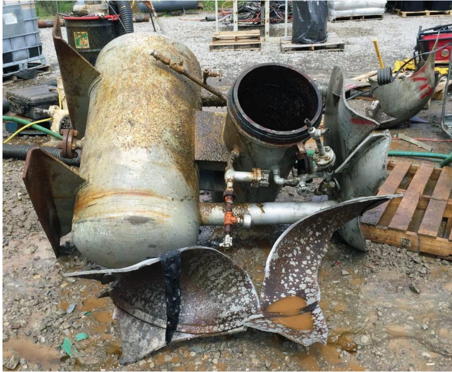
Figure 10. MP Odorizer That Exploded on May 24, 2017. This photo shows the failed MP odorizer from the May 24, 2017, explosion. (Credit: MRR).
