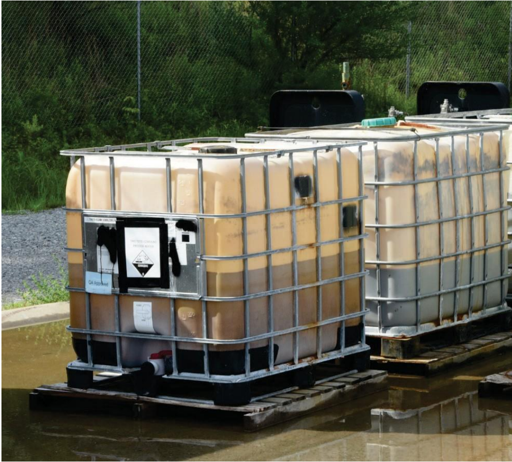
Figure 5. Process Water Totes. This picture shows totes at MRR containing “process water” that MRR technicians have pumped out of treated odorizer equipment. (Credit: CSB).
