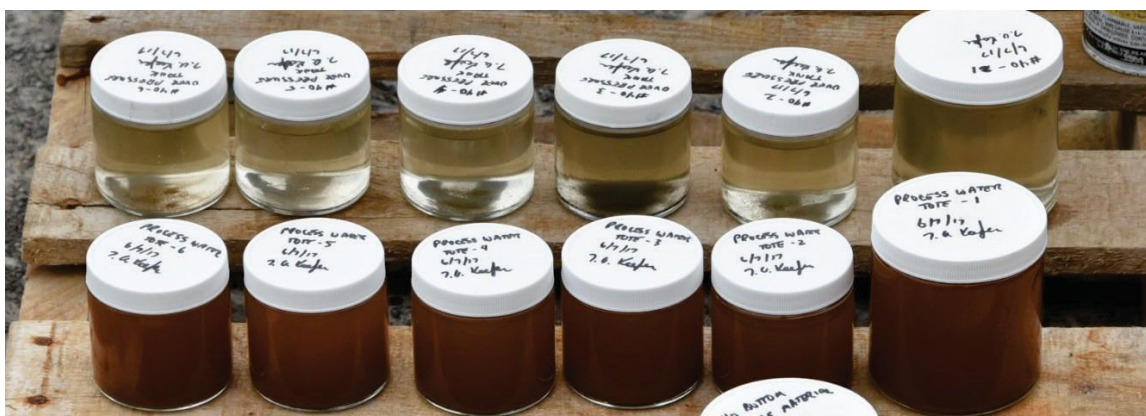
Figure 12. Process Water. The light-yellow samples (top row) were taken from the bottom chamber of the MP odorizer that exploded on May 24, 2017. The brown samples (bottom row) were taken from a “process water” tote not involved in the May 24, 2017, incident. Note the color differences showing the drastic color variation of the process water, indicating that different vessels likely had different types and quantities of materials in them before chemical treatment. (Credit: CSB).
