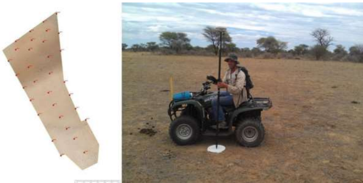
Figure 5. Using an ATV and RTK GNSS to place and survey 32 GCPs
