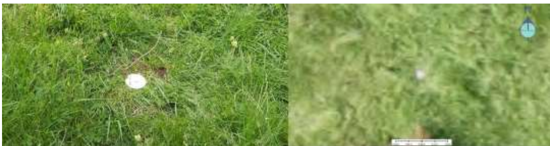
Figure 14. Pre-marked survey point consisting of a round white 10 cm disc, left as seen from eye level and right as projected in the orthophoto.
