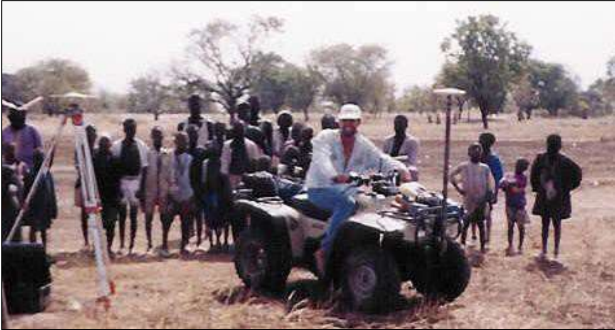
Figure 8. Typical GNSS PPK base station and rover setup for large area terrestrial ATV-supported terrain modelling methods
