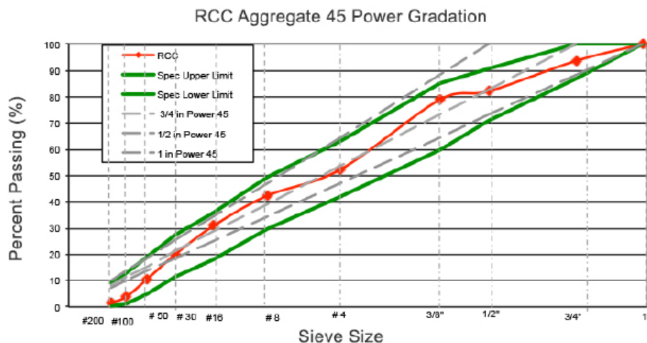
Figure 1. Example RCC concrete gradation.
