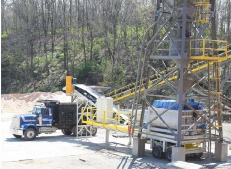
Figure 6. Twin shaft horizontal mixer—batch type.
