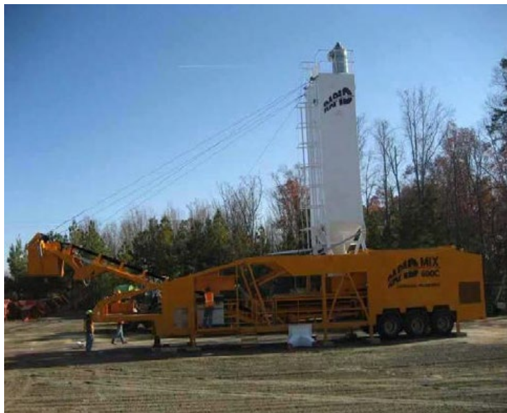
Figure 7. Twin shaft horizontal mixer—continuous type.
