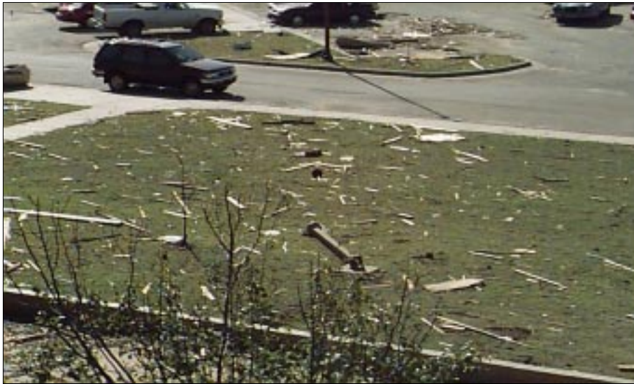
FIGURE 3-23: Wood framing members and plywood sheathing near the periphery of a violent tornado damage area in Moore, Oklahoma, displaying quantity of flying debris.
