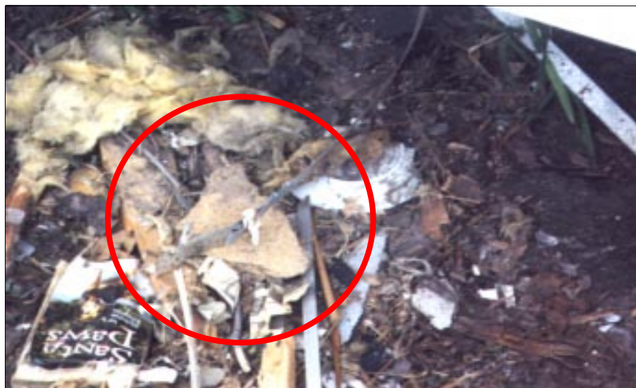
Figure 4-53: Strap torn off from chassis of manufactured home. This home in Wichita, Kansas, was located within the inflow area of a severe tornado.
