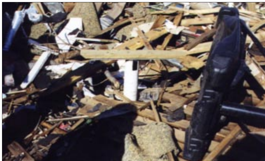
FIGURE 6-18: Heavy gauge ventilation pipe for a below ground shelter in Oklahoma withstood considerable debris impact.
