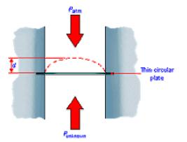
Because the displacement of the diaphragm is small, a displacement sensing device with high resolution, sensitivity and accuracy is required. Also, a non-contact device is required as any mechanical resistance will reduce the displacement even more. Using the diaphragm as one plate
