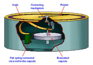
capsule flattens. If atmospheric pressure rises, the capsule expands. This displacement is detected
