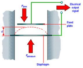
An electrical signal is connected to the two plates of the capacitor. The change in value of the capacitance causes this electrical signal to vary. This is then conditioned and displayed on a device calibrated in terms of pressure.
