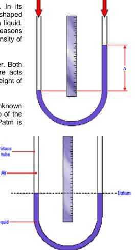
g is the acceleration due to gravity, that is, 9.81 m.s<sup>-2</sup> h is difference between the heights of the liquid in each limb, in m
