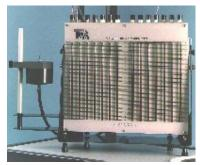
Inclined tube manometers are used where higher sensitivity than a U-tube manometer is required. It cannot be read remotely, and it is usually used with gases.
