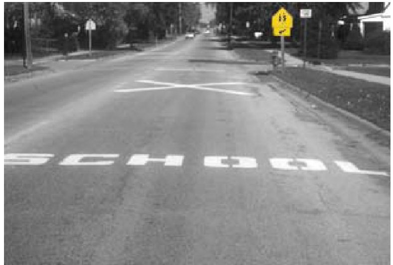
Pavement markings convey important information to drivers without diverting their attention from the road.
