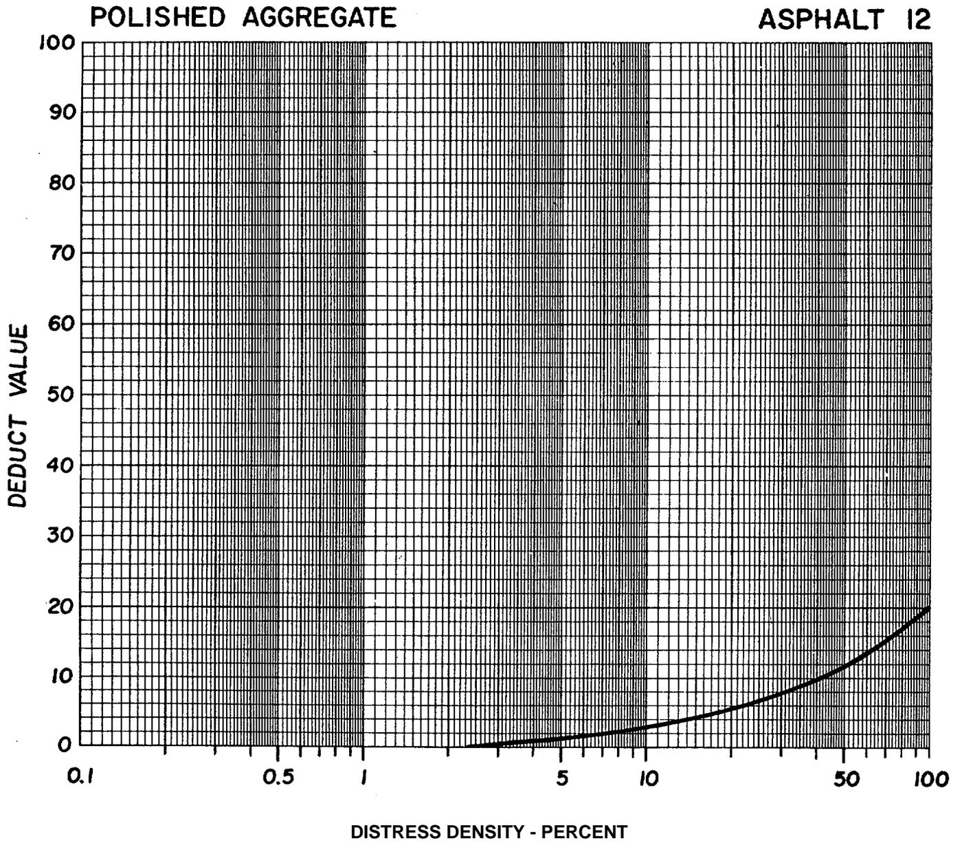
Figure C-12. Deduct value curves for polished aggregate.
