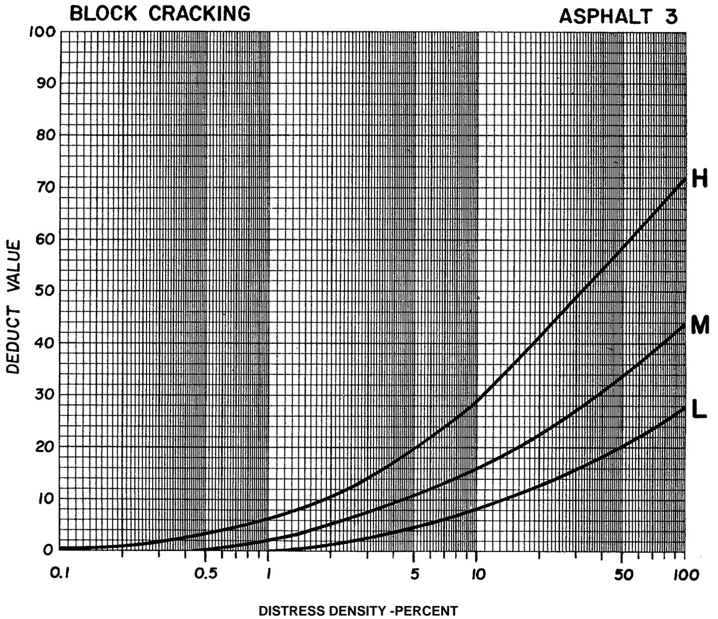
Figure C-3. Deduct value curves for block cracking.
