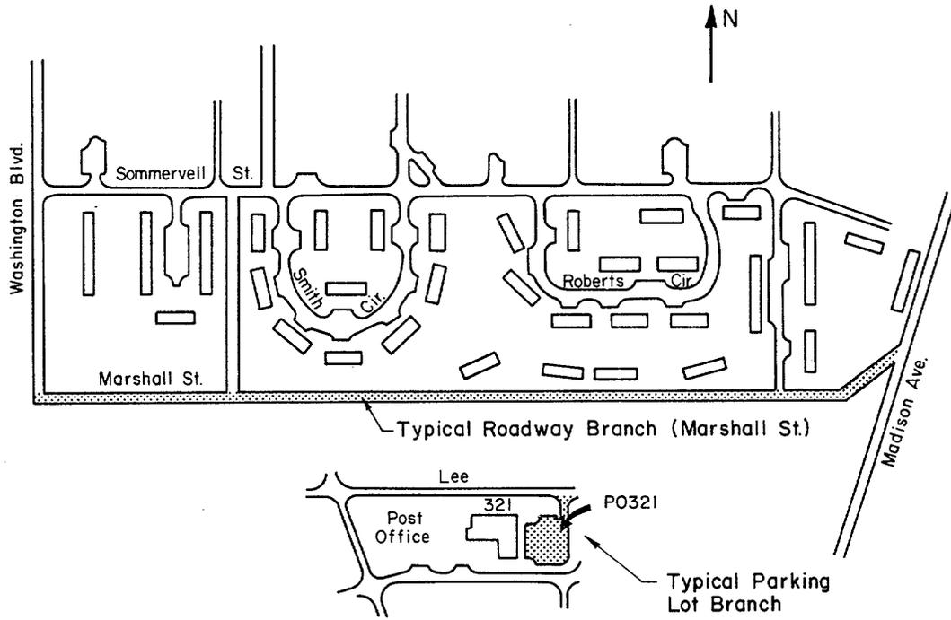
Figure 2-1. Installation map showing typical pavement branches.
