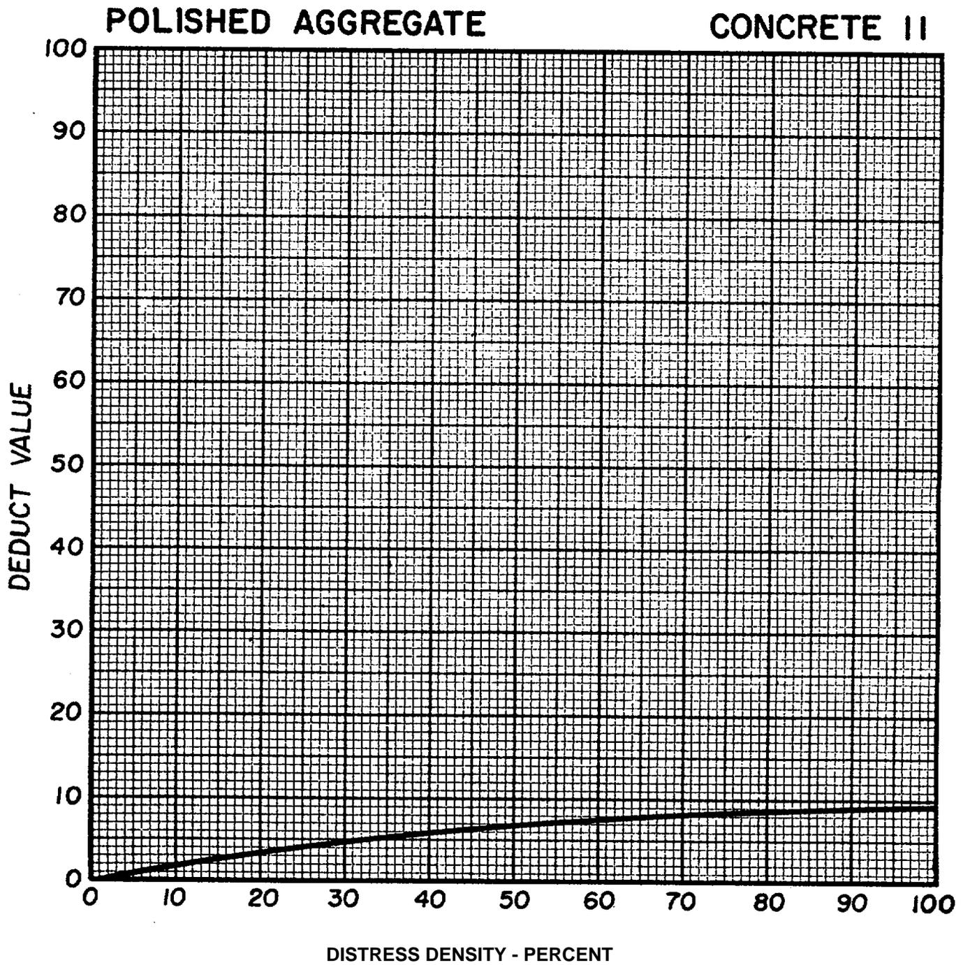
Figure C-31. Deduct value curve for polished aggregate.
