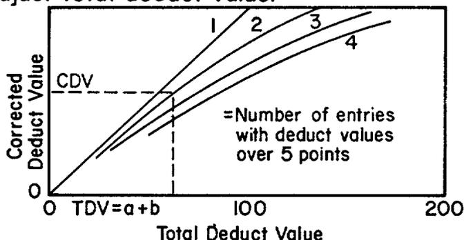
**Step 5. Compute pavement condition index (PCI) = 100 - CDV for each sample unit inspected**
