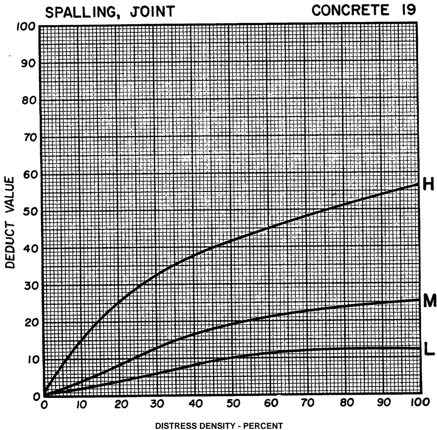
Figure C-39. Deduct value curves for spalling, joint.
