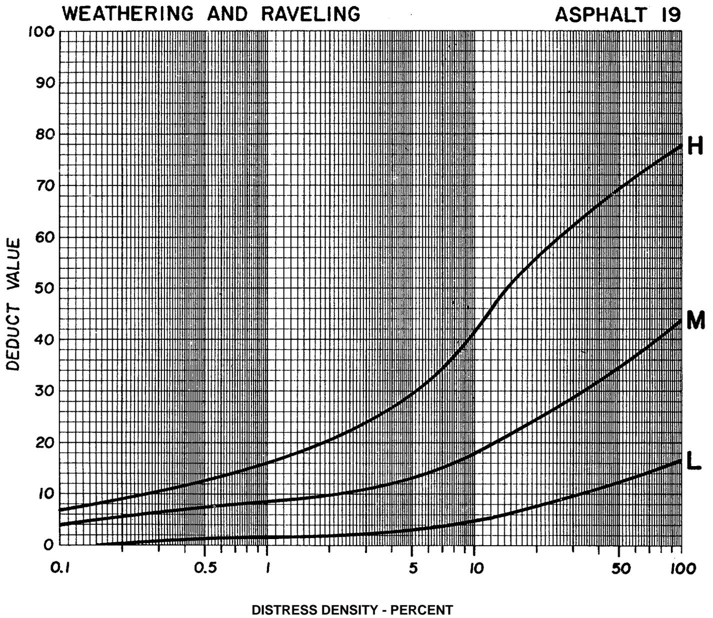
Figure C-19. Deduct value curves for weathering and raveling.
