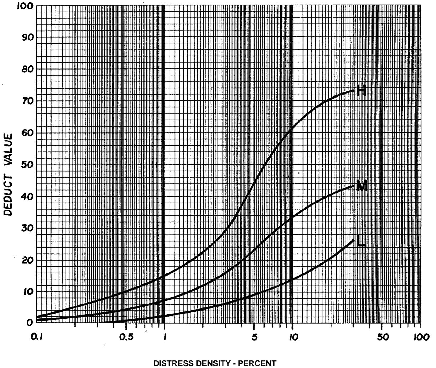
Figure C-8. Deduct value curves for joint reflection cracking.
