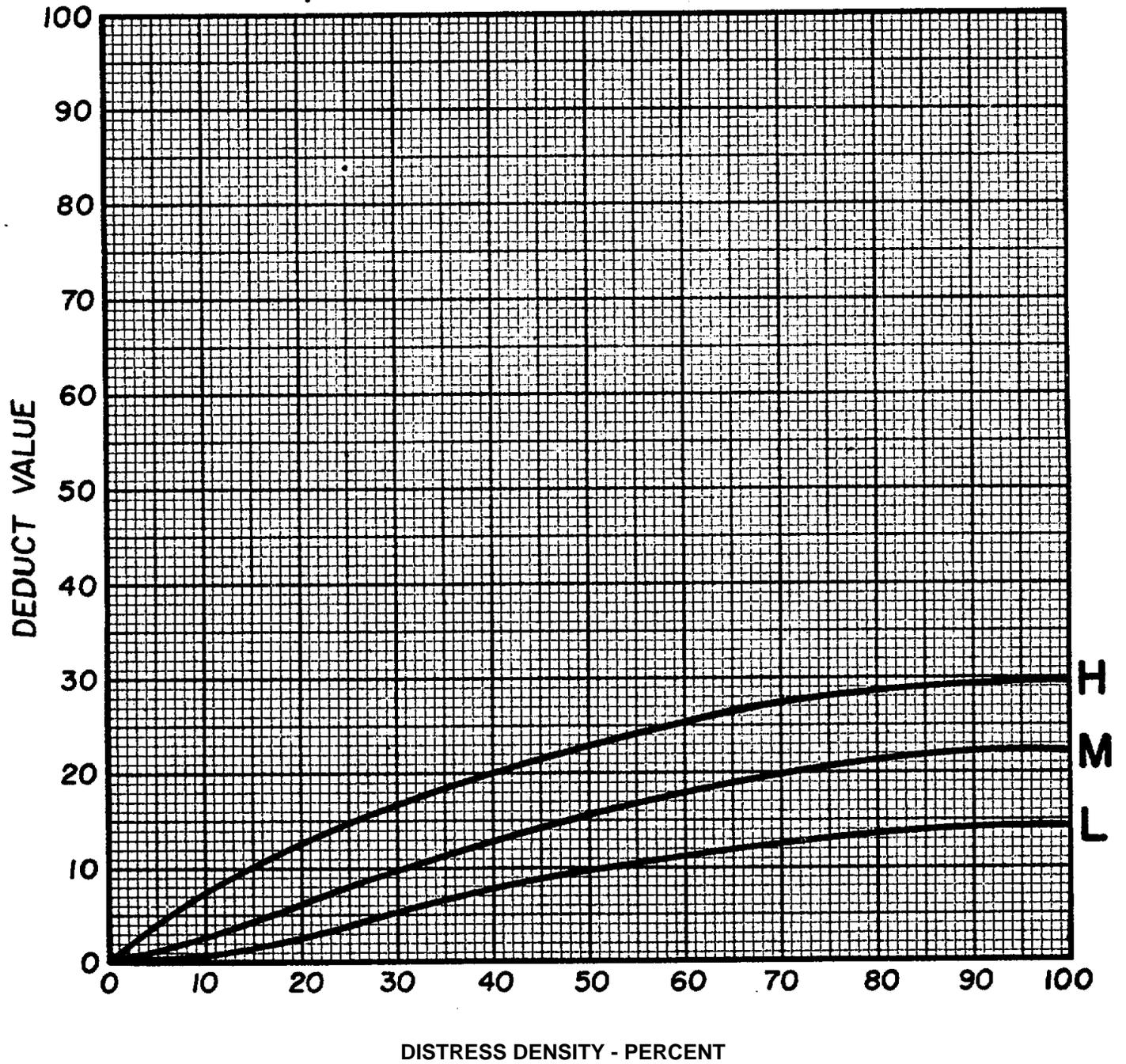
Figure C-38. Deduct value curves for spalling, corner.
