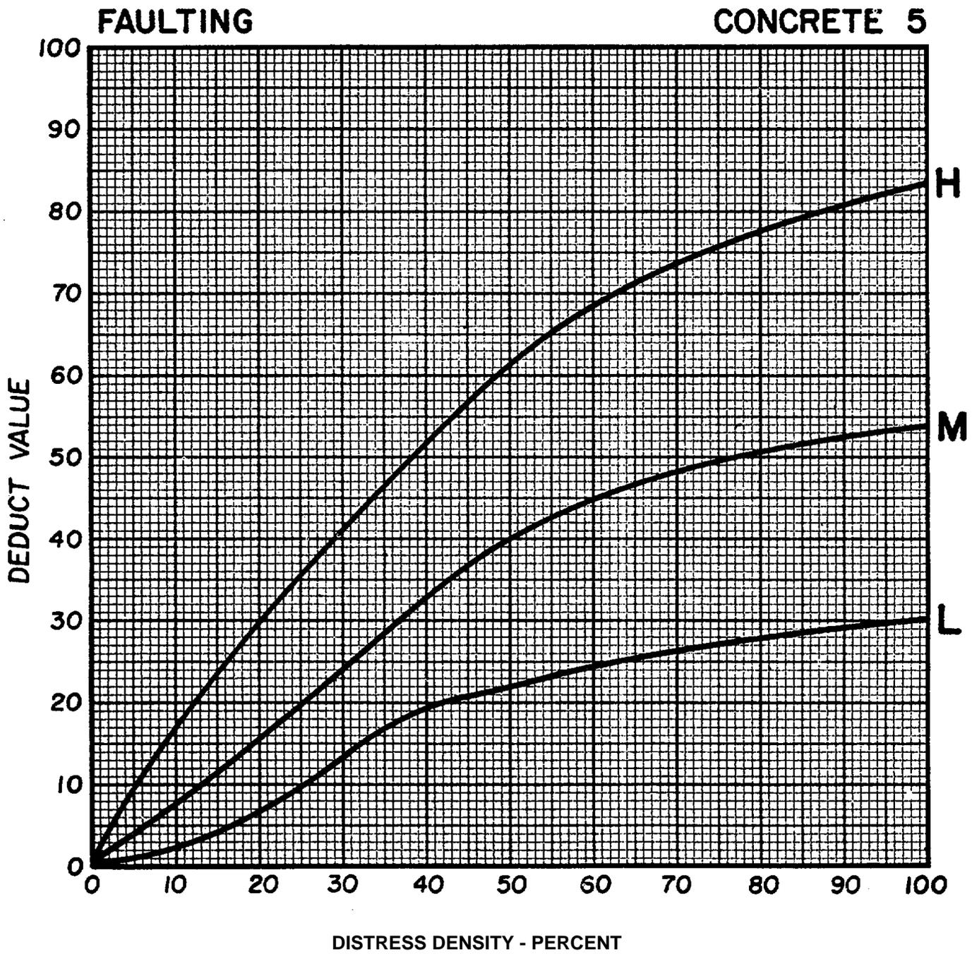
Figure C-25. Deduct value curves for faulting.
