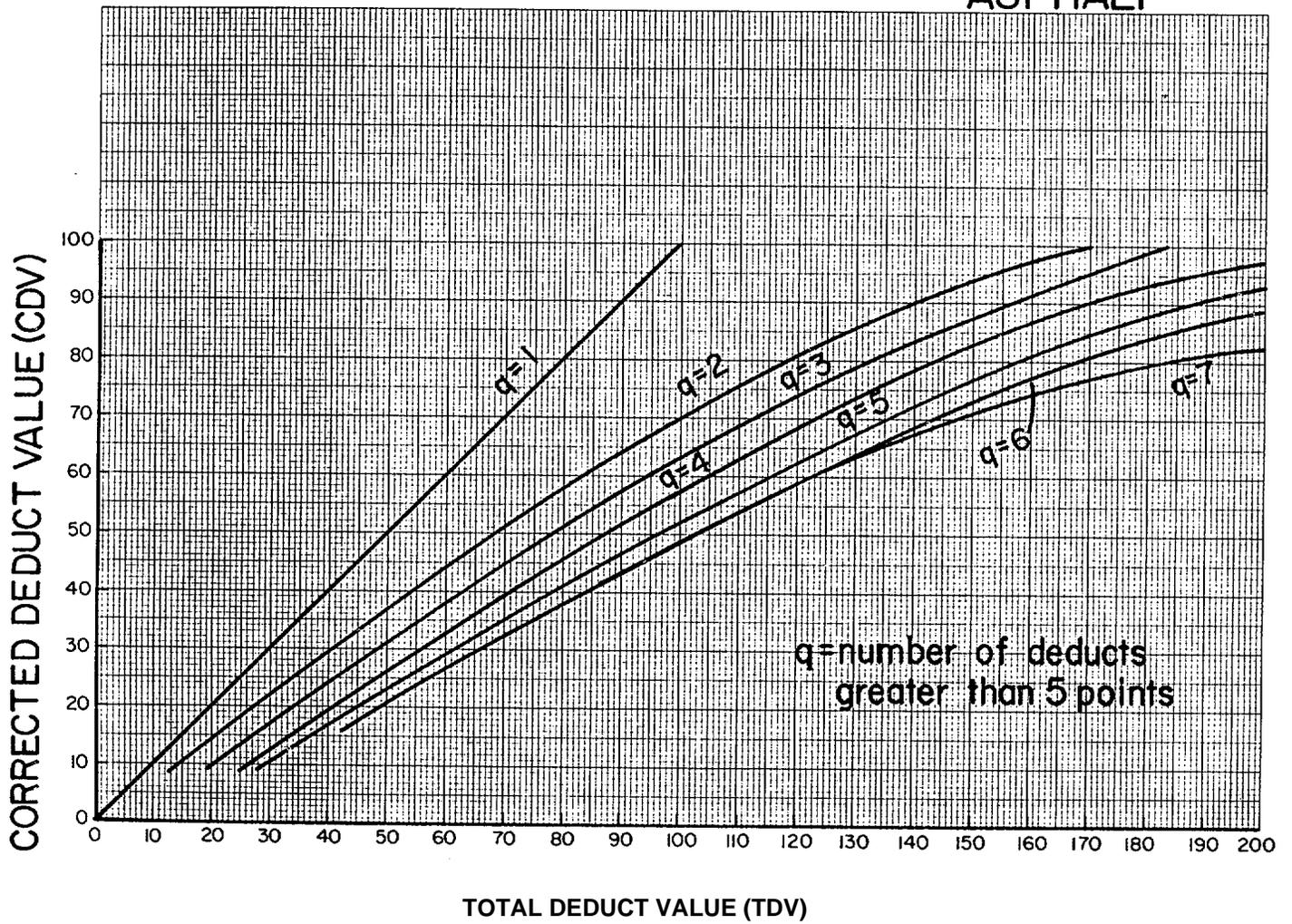
Figure C-20. Corrected deduct value curves for asphalt-surfaced pavements.
