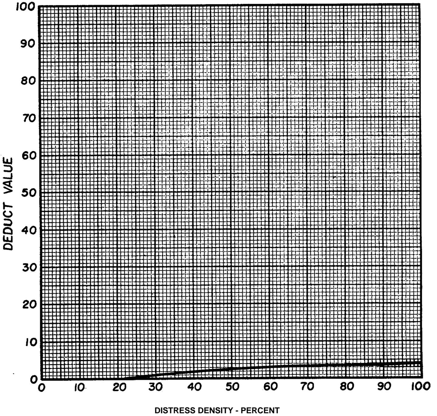
Figure C-37. Deduct value curve for shrinkage cracks.
