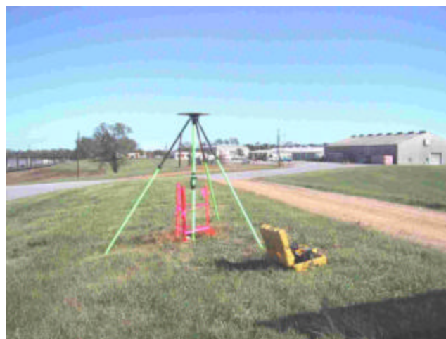
Figure 6-1. Control survey observing scheme on Mississippi River and control point baseline occupation at Memphis District Ensley Boatyard (Memphis District and 3001, Inc.)
