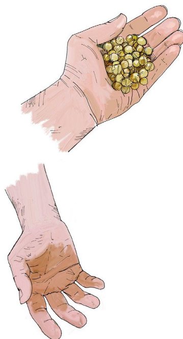
Figure 4. If your hand is stained with aggregate, consider washing the aggregate again
