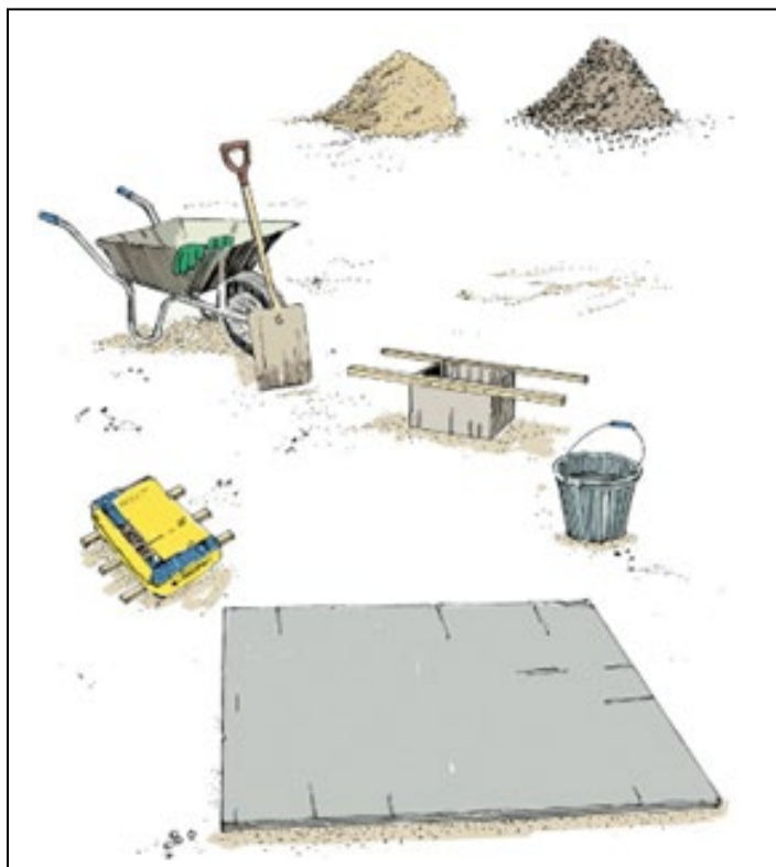
Figure 7. Materials and equipment required for handmixing concrete
