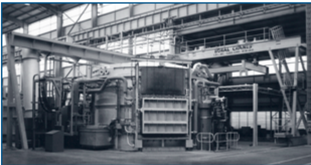
Tiling Top Aluminum Melting Furnace
