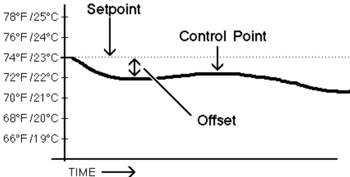
**Offset** is the amount away from setpoint, or the difference between the Setpoint and the Control Point. In the example above, the offset is approximately 2°F (1°C).
