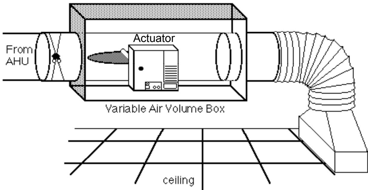
The VAV box has a **Damper** that modulates to maintain the space temperature by increasing or decreasing the volume of air being delivered to the space. The airflow is measured in [\*cubic feet per minute \(CFM\)\*](#) or *liters per second (L/s)*. If the space is too warm, the damper is adjusted to allow more 55°F (13°C) air into the space. If the space is too cool, less air is delivered to the space.
