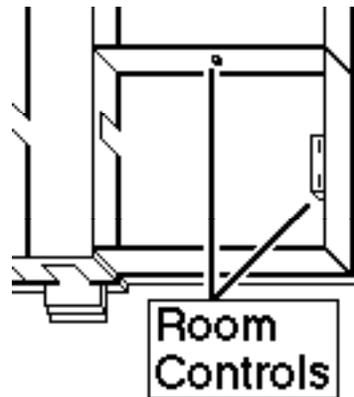
One way to control the temperature in a room is with a **Wall Thermostat** (stat) that sends a signal to an actuator that positions a damper to modulate the airflow in a *variable air volume* (VAV) box. These VAV boxes are installed in the space between the ceiling tile and the structural ceiling. This space is sometimes used as a return air *plenum*, as part of the *building air distribution system*.
