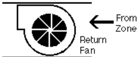
The supply air fan distributes the air into the rooms or zones. After the air has gone through the zones, it comes back to the **Return Fan**, which routes the return air back to the return air dampers or the exhaust air dampers.
