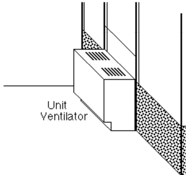
A **Unit Ventilator**, common in schools, is shown above. It serves as the local air-handling unit and has dampers for the outside and return air, a fan, and a hot water coil. The hot water comes from the boiler. The diffusers are on the top of the unit. A space thermostat controls the valve and dampers in this unit. A switch on the base of the thermostat starts the fan inside the unit ventilator.
