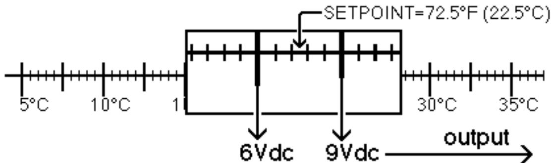
A signal from the sensor is sent to the controller. In this example, 72.5°F (22.5°C) is the setpoint or desired temperature for a room.
