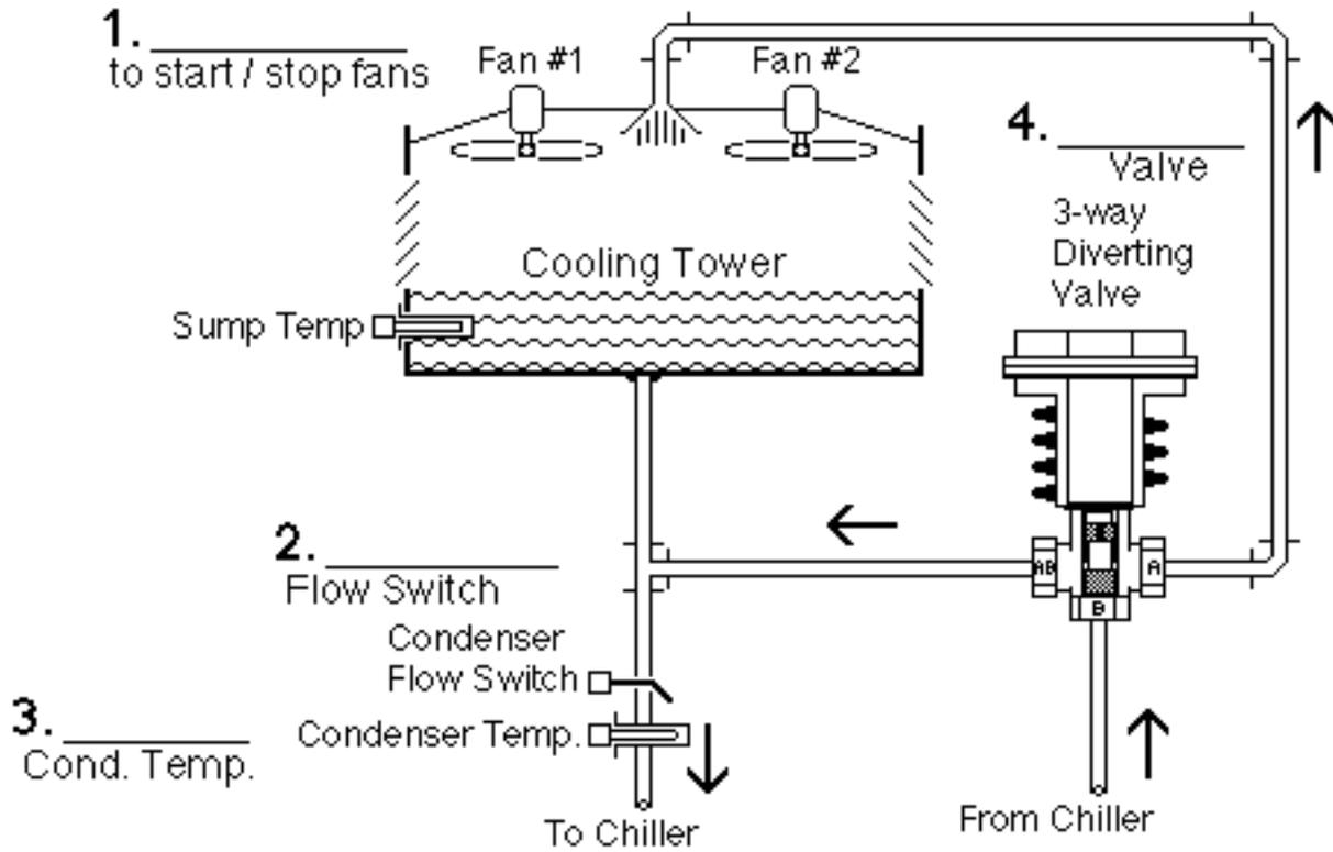
Identify the numbered points in the following diagram as either: **AI**, **DI**, **AO**, or **DO**
