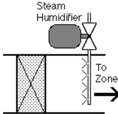
A steam **Humidifier**, or some other form of humidifier, is placed inside an AHU to add moisture to the air when needed. Humidity levels, sensed in the return air, are set at 35% RH, for example. The two-way normally closed (N.C.) valve is modulated to maintain 35% RH, plus or minus an acceptable tolerance.
