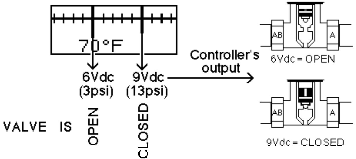
As an example of an electronic controller connected to a transducer, 6 Vdc is converted into 3 psig, causing the valve to be open. At 9 Vdc, the output from a transducer is 13 psig, completely closing the valve. With a pneumatic controller, 3 psig is sent to the actuator, completely opening the valve. When the controller sends a 13-psig signal to the actuator, the valve strokes to the completely closed position.
