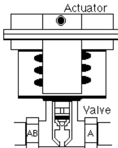
This actuator operates with either a pneumatic controller or with an electronic controller which sends its signal through a *transducer*.
