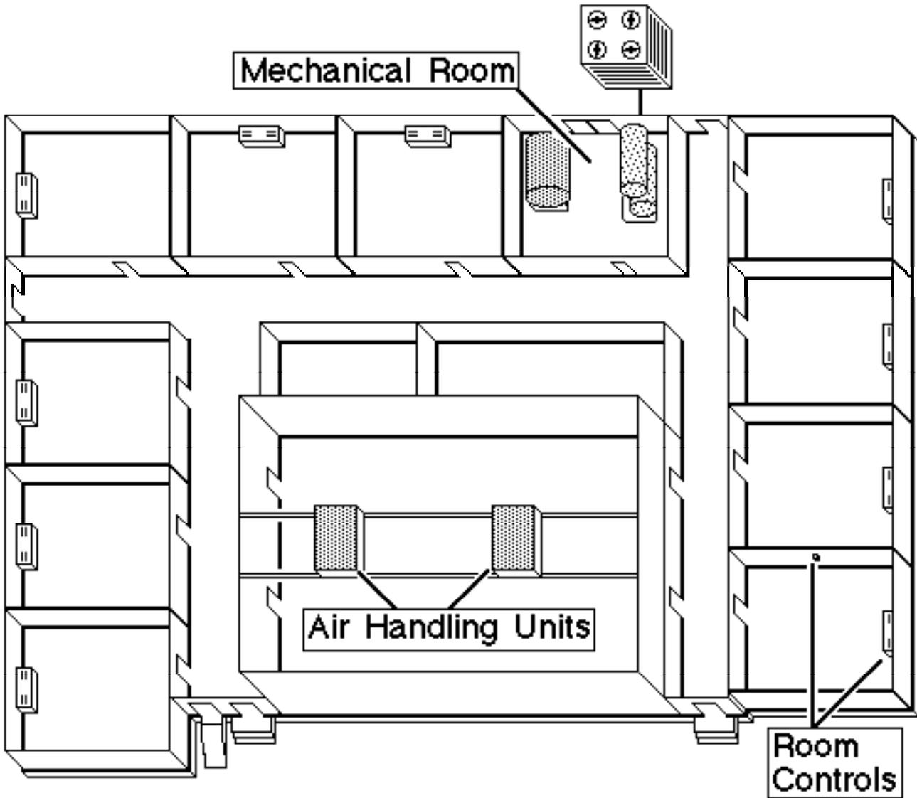
**Mechanical Room:** Boilers, chillers, pumps, heat exchangers, and other associated equipment are found inside the mechanical room. This area is sometimes called the main equipment room.
