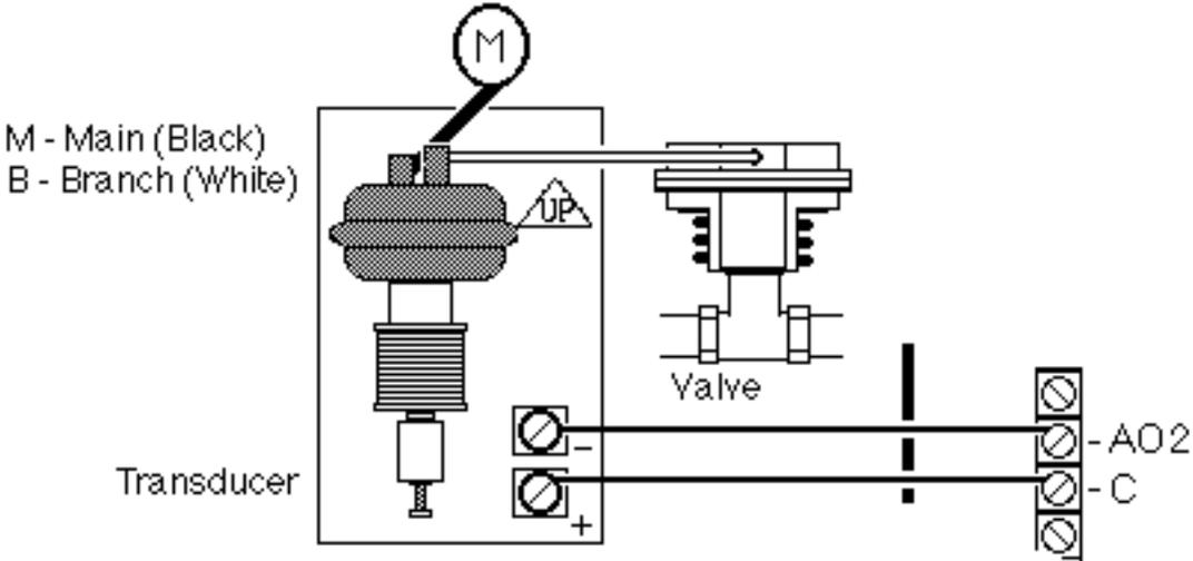
Another E-P transducer converts a 4 to 20 mA current signal to a 3 to 15 psig pneumatic signal. Setup is required on this transducer also, to adjust the current signal to the desired pneumatic output signal.
