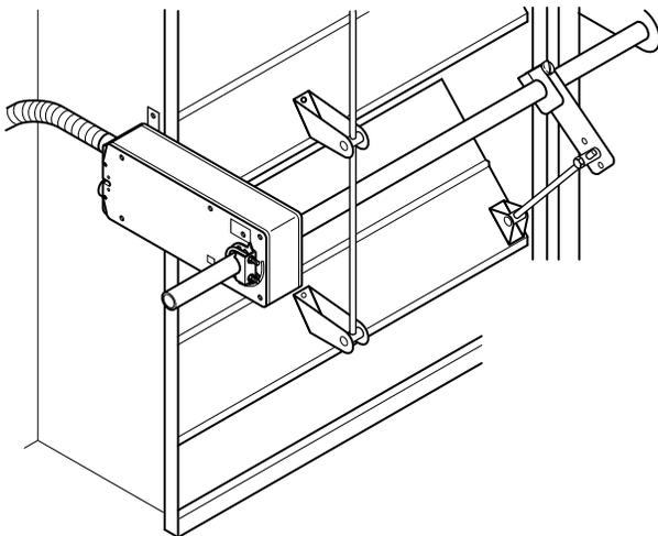
? When used on dampers, direct-coupled DuraDrive™ actuators require minimal or no external linkage, making installation easy to perform. DuraDrive actuators may also be used with ball and globe valves, and are also available as complete actuator and valve assemblies. They are manufactured in a variety of models, including [spring-return](#), non-spring return, two-position, proportional, and floating control.
