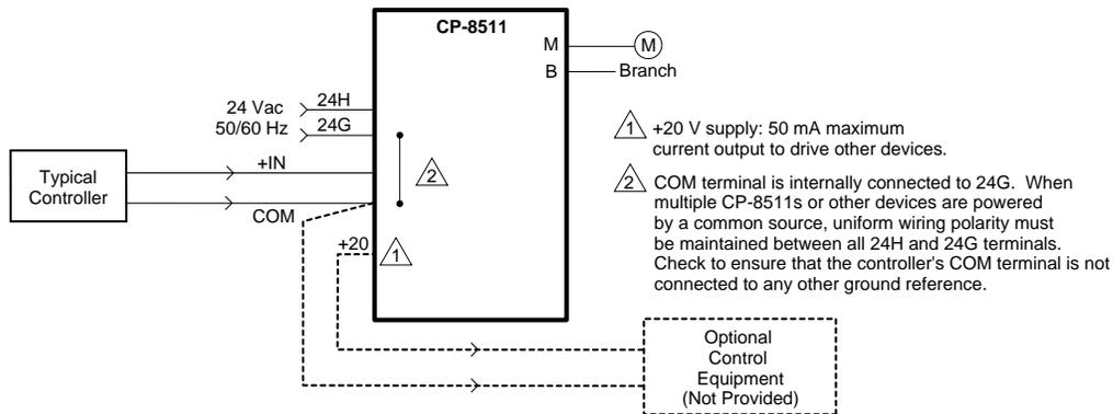
Figure 1 Typical CP-8511 Wiring with Optional +20 Vdc Supply.
