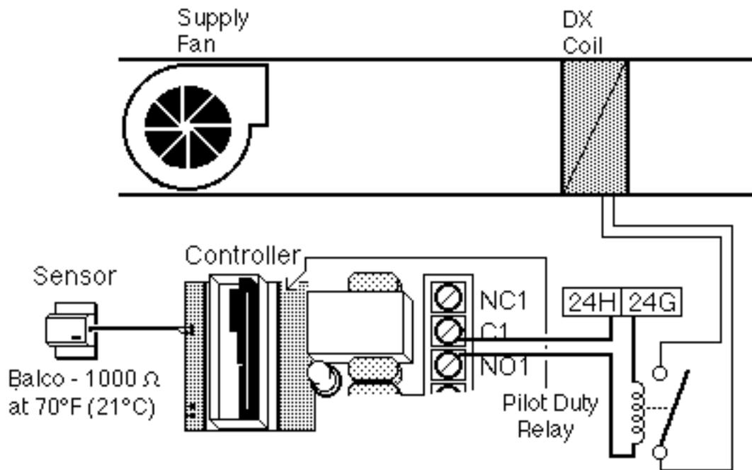
In the above example, when the room temperature rises, the controller sends a signal to close the pilot duty relay. The normally open contact is then made to common. This completes the circuit and starts the DX cooling. When the temperature drops, the controller returns the relay output to its open (normal) position, thereby turning OFF the DX cooling.
