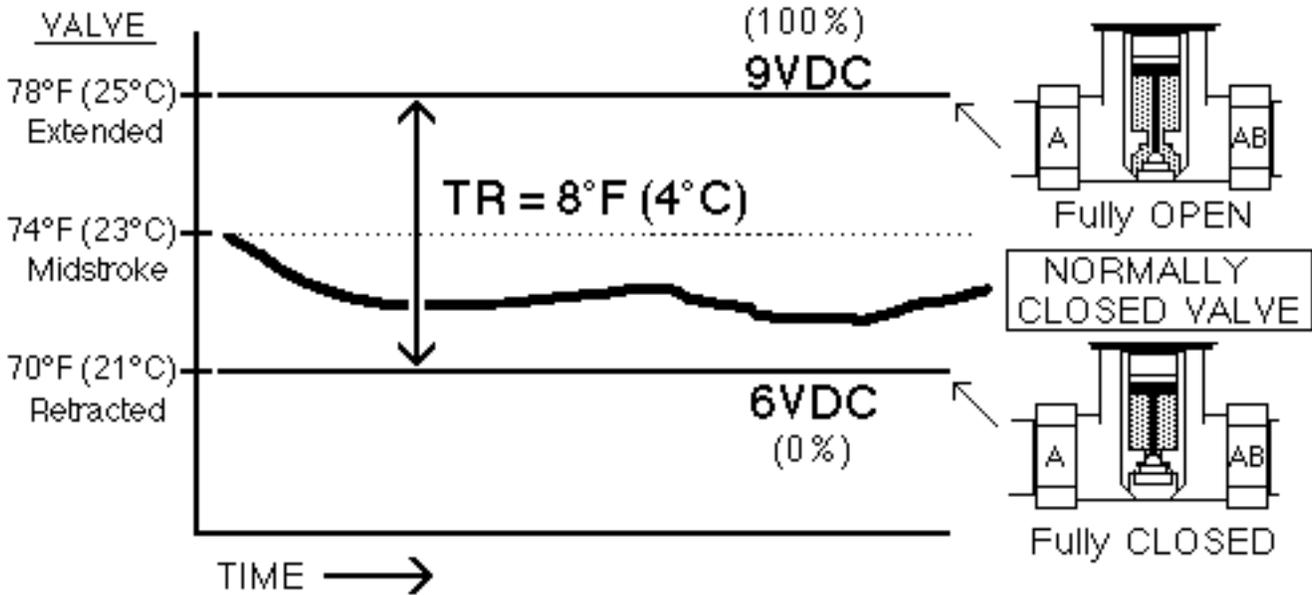
Throttling range is sometimes referred to as “sensitivity”. Typical throttling ranges are 8° to 10°F (4° to 5°C) for mechanical controls such as mixed air control and the control of hot water supply. In contrast, room controls must be much tighter, with a throttling range between 2° and 4°F (1° to 2°C)
