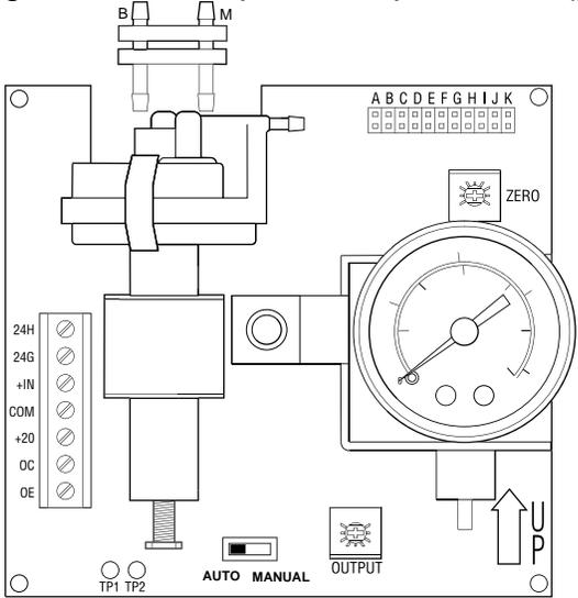
A voltage transducer may convert a 0 to 5 Vdc, 0 to 10 Vdc, or 1 to 11 Vdc signal to a pneumatic signal from 3 to 15 psig. Setup is required to modify the voltage signal to match the desired pneumatic output signal.
