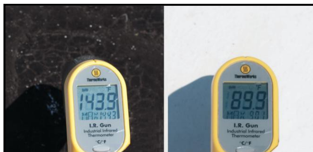
Figure 1: Dark vs. Cool Roof Surface Temperatures
