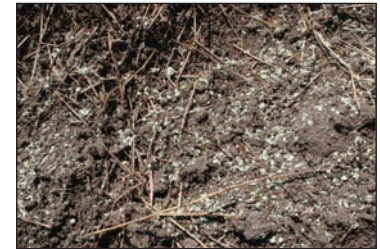
Figure 18: PAM flocculent on soil
