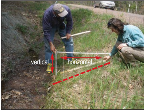
Figure 42: Ditch front slope example
