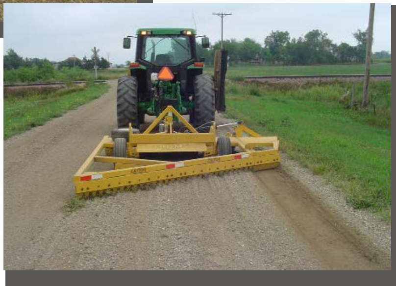
Example of a light blading device being towed by a mower tractor.
