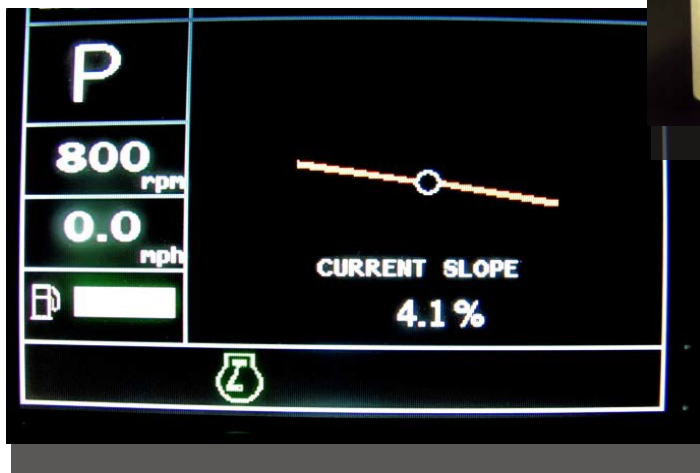
Two examples of screens in the grader cab showing electronic slope controls being used to construct at or near 4 percent crown, or cross-slope, on the road surface.
