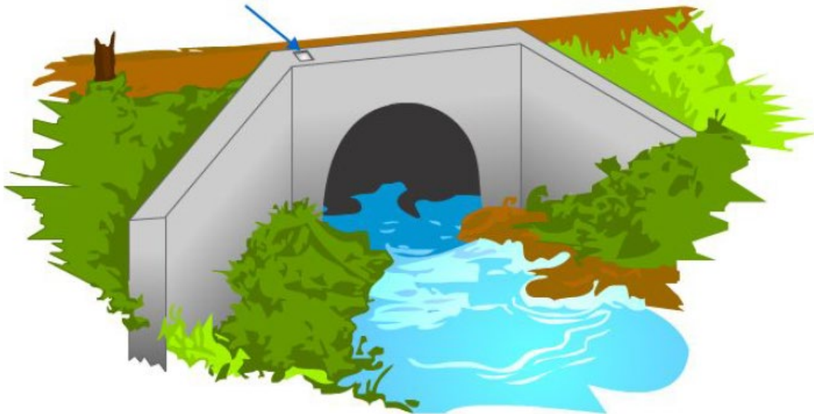
Figure 2 – Points on existing structures used as bench marks.
