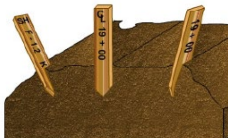
Figure 38 – Center line and shoulder stakes.
