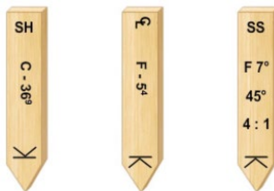
Figure 33 – Combined alignment and grade stakes.
