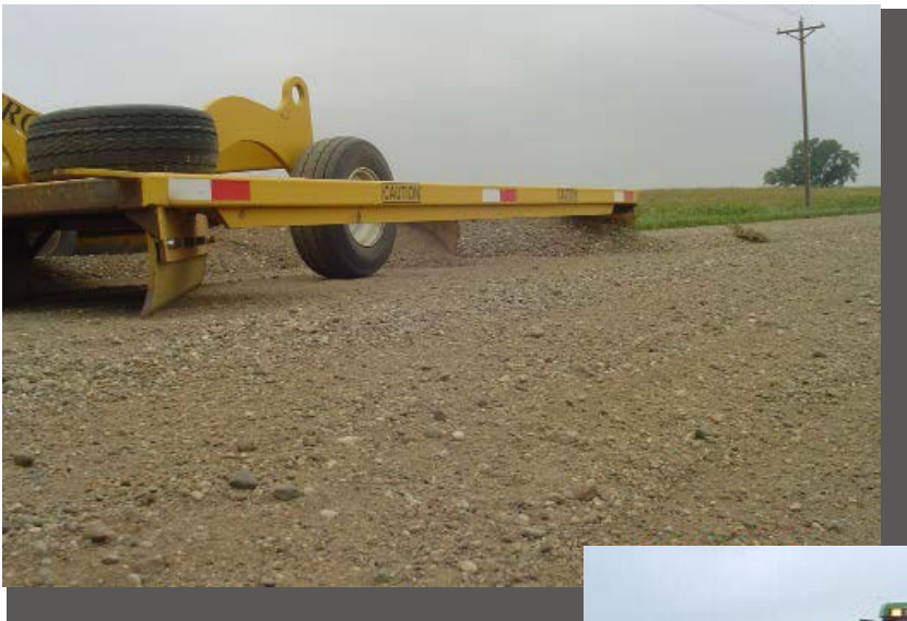
Example of a light blading device being towed by a mower tractor.
