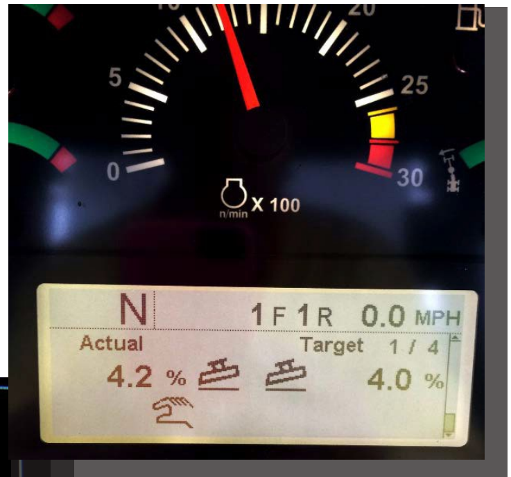
Two examples of screens in the grader cab showing electronic slope controls being used to construct at or near 4 percent crown, or cross-slope, on the road surface.
