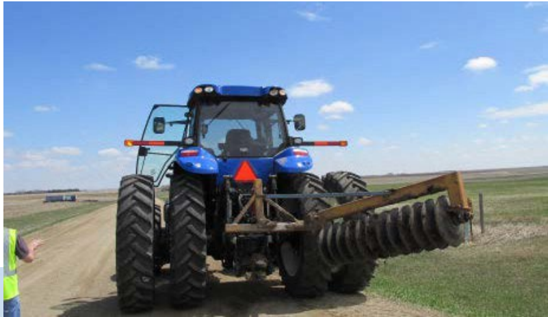
Example of a shouldering disk mounted on a tractor to process sod and gravel before moving it back to the road.
