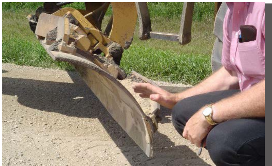
Trainer is demonstrating correct pitch of moldboard for most maintenance operations.
