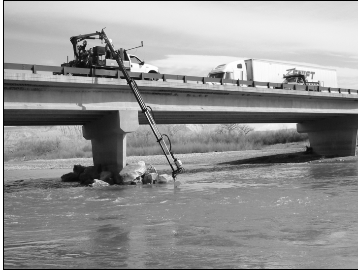
Figure 9.9. Sonar instrument deployed from articulated arm truck.
