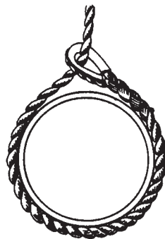
Correct – Use thimbles in the eyes.
