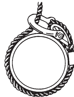
Correct – Shackle pin cannot turn.
