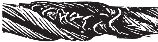
Rope that has been jammed after jumping off sheave
