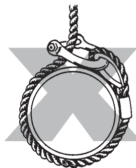
Incorrect – Shackle pin bearing on running line can work loose.
