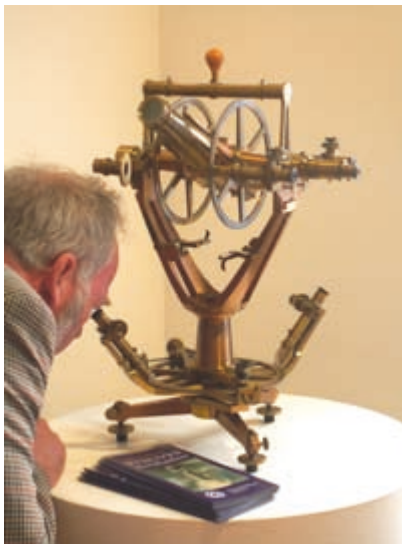
A recently re-discovered Repsold theodolite used on the Struve Arc.
