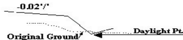
**Figure 15-4 Daylighting Example**
