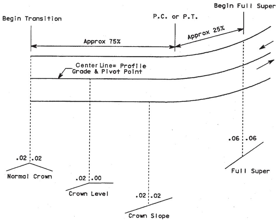
**Superelevation for Two-Lane Highway**
