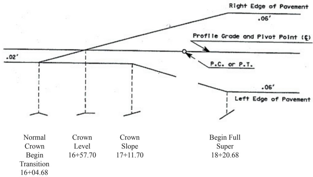
**Superelevation Diagram for Two-Lane Highway**
