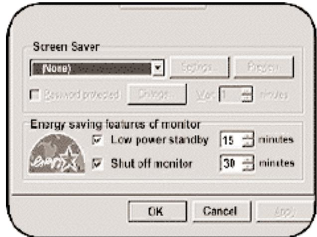
Energy Star monitors allow the user to set low power and power-off timing via software.
