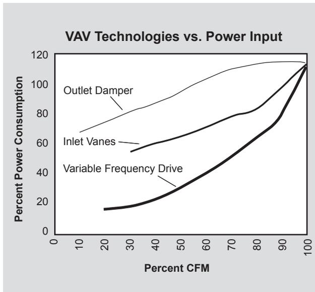
On existing VAV systems, convert airflow control from inlet vanes or outlet dampers to variable frequency drives (VFDs). Notice on the graph above how energy consumption using VFDs is far lower than using outlet dampers or inlet vanes.
