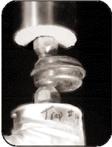
Traps subject to freezing temperatures may be damaged by water held inside the trap when the steam system is shut down. Replace traps subject to freeze damage with self-draining types.
