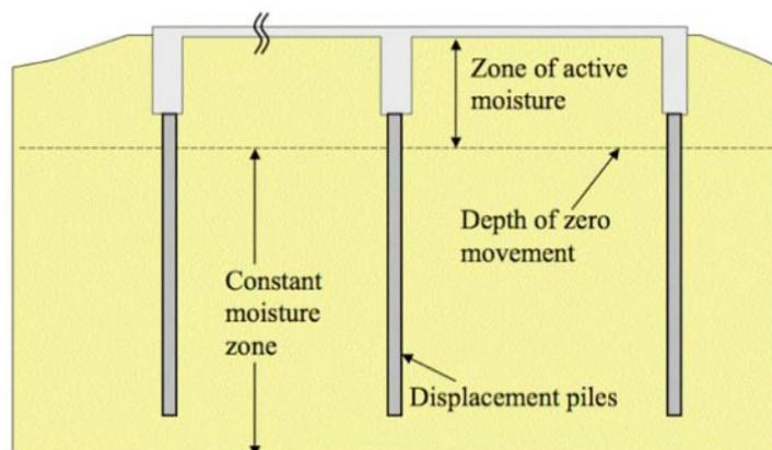
**Figure 5.1.4 Displacement Piles**
