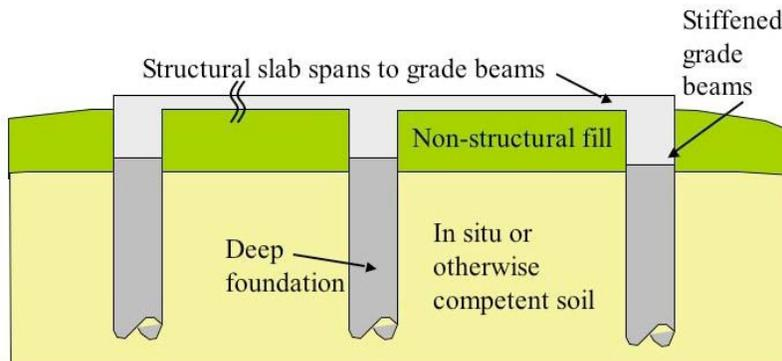
**Figure 4.1.2 Stiffened Structural Slab with Deep Foundations**
