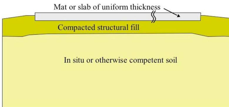
**Figure 4.2.3 Grade-Supported Non-Stiffened Slab of Uniform Thickness**
