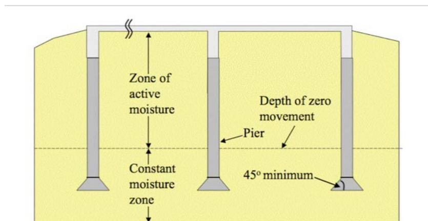
**Figure 5.1.1 Drilled and Underreamed Concrete Piers**
