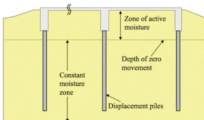
**Figure 5.1.4 Displacement Piles**
