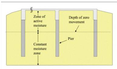
Figure 5.1.2 Drilled Straight-Shaft Concrete Piers
