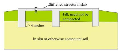
Figure 4.2.1 Grade-Supported Stiffened Structural Slab
