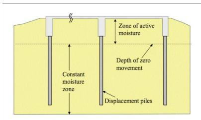
Figure 5.1.4 Displacement Piles
