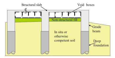
Figure 4.1.1.1 Structural Slab with Void Space and Deep Foundations
