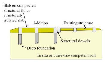
Figure 4.3.2 Mixed Depth System for Building Addition with Deep Foundations
