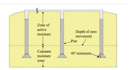
Figure 5.1.1 Drilled and Underreamed Concrete Piers
