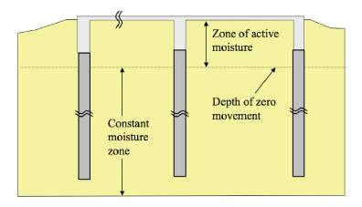
Figure 5.1.3 Auger-Cast Concrete Piles
