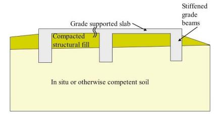
Figure 4.2.2 Grade-Supported Stiffened Non-Structural Slab
