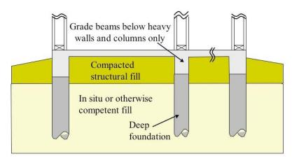
Figure 4.1.4 Non-Stiffened Slab-on-Grade with Deep Foundations
