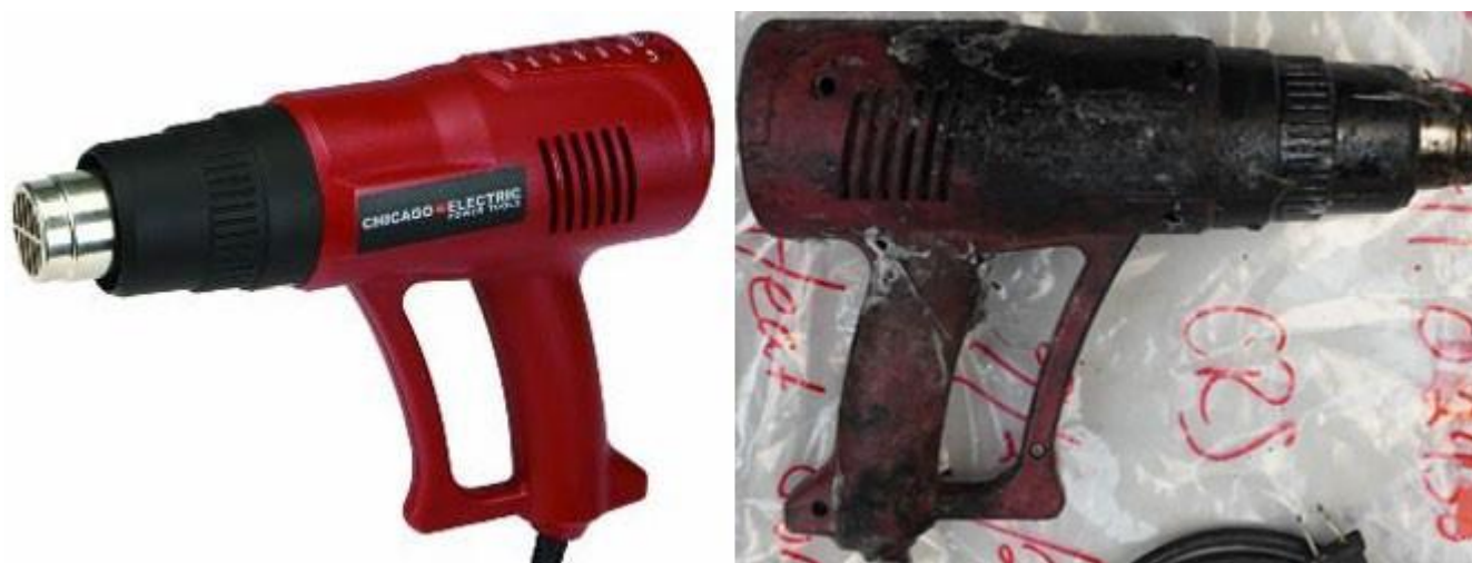
Figure 4. Exemplar heat gun (left). Heat gun recovered from scene (right). (Credit: Harbor Freight [6], CSB.)
