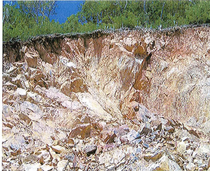
Figure 19. Close-up View of Figure 17 Showing a Rock Block Sled away, Looking Toward West.
