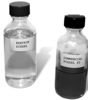
*Zero sulfur, zero aromatics, high cetane diesel fuel made by Rentech, Inc., a small fuel development company based in Denver, Colorado.*
