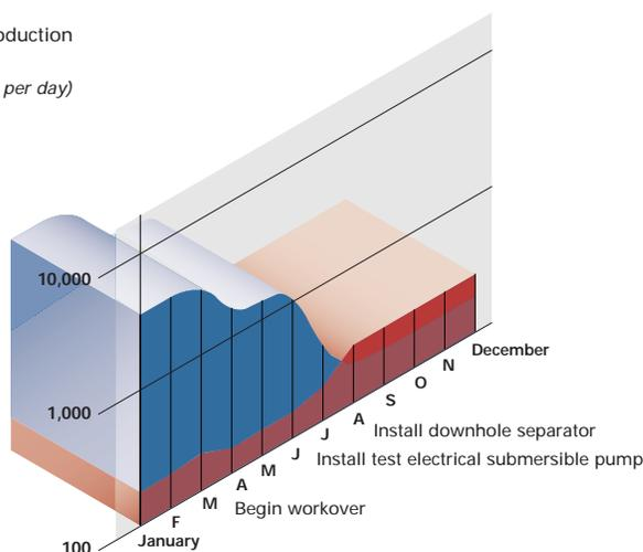
Currently being tested in pilot-scale projects throughout the world, downhole separation may someday deliver significant cost savings and environmental benefits in settings where the technology is applicable. In one recent demonstration (illustrated here), downhole separation decreased surface water production by 95 percent and increased oil production by 50 percent, resulting in a 4-month payback period.
