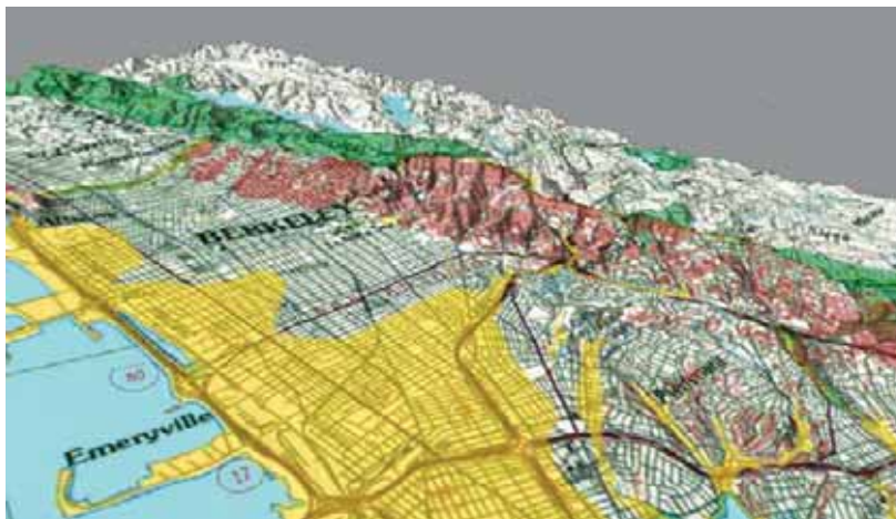
Figure 3-12: 3-D image of Liquefaction and Landslide Hazard Zone Map for Berkeley and Emeryville. Yellow indicates liquefaction, which is related to soil type and proximity to ground water.
