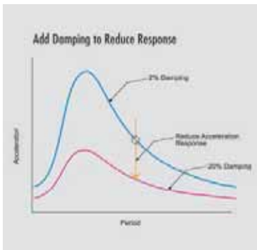
Figure 7-17: Reduction of demand by damping.
