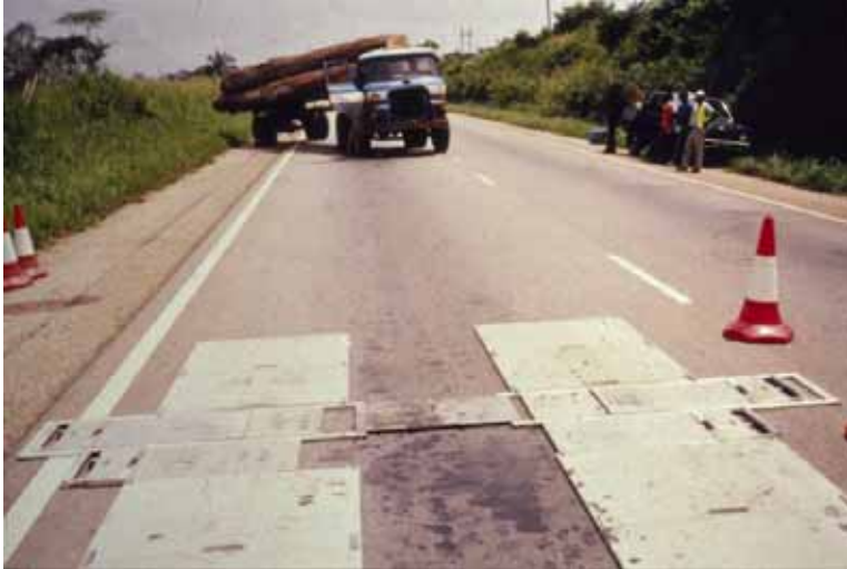
Figure 51: Simple axle load unit as used for surveys in Ghana
