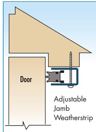
**Adjustable jamb/head weatherstripping:** This type of weatherstripping is recommended because the wide sponge neoprene offers good contact with the door (see Figure 4-42). The adjustment feature also helps to ensure good contact, provided the proper adjustment is maintained.
