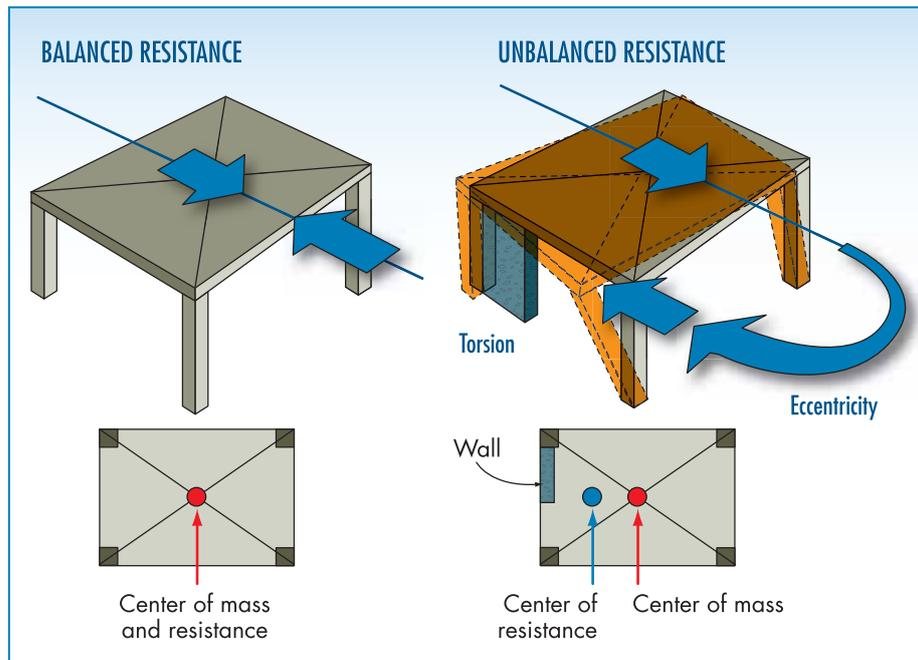
One building configuration that is most likely to produce torsion features re-entrant corners (buildings shaped in plan like an “L” or a “T,” for example). The wings of such buildings tend to twist and result in torsion and stress concentration at the “notch” where the wings meet, also called a re-entrant corner (Figure 2-13).
