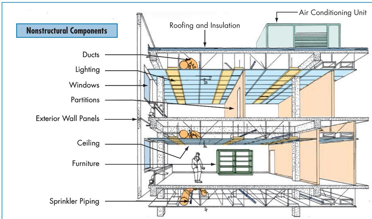
Figure 2-15b: Structural and nonstructural elements of a building
