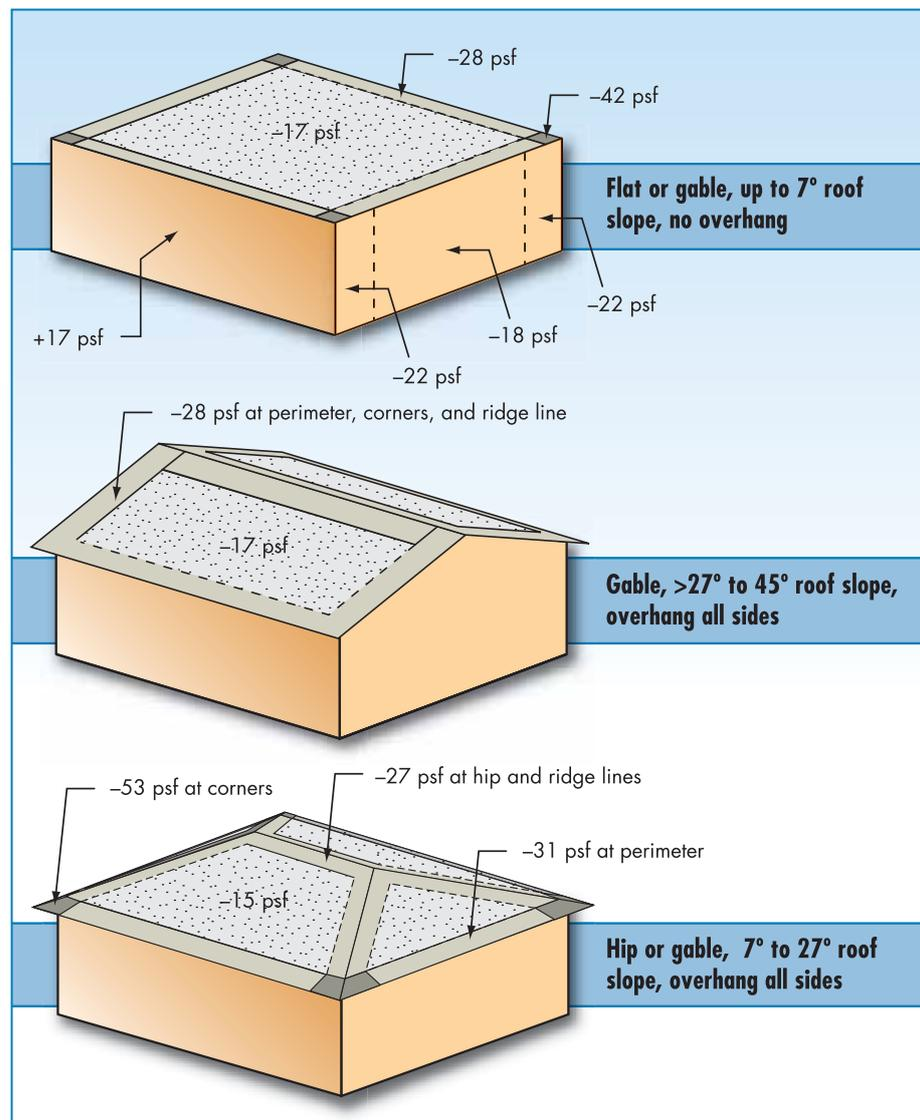
Aerodynamic influences are accounted for by using external pressure coefficients in load calculations. The value of the coefficient is a function of the location on the building (e.g., roof corner or field of roof) and building shape as discussed below. Positive coefficients represent a positive (inward-acting) pressure, and negative coefficients represent negative (outward-acting [suction]) pressure. External pressure coefficients for MWFRS and C&C are listed in ASCE 7.
