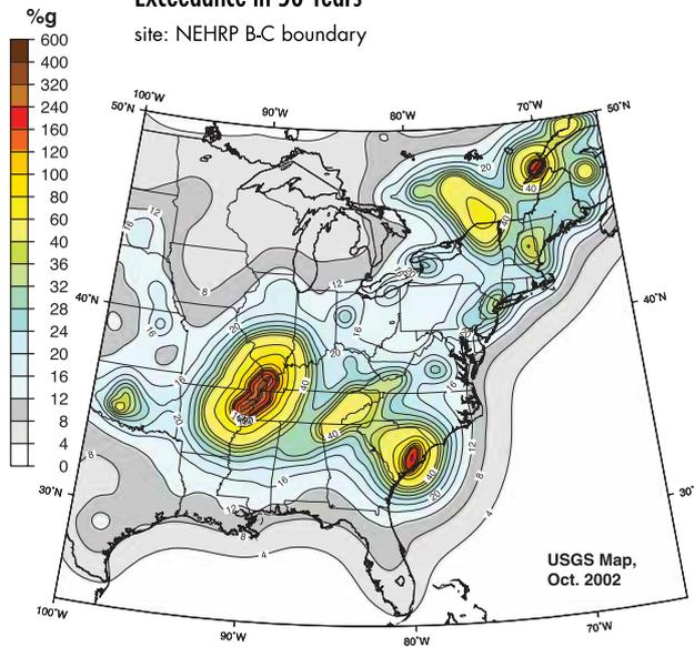
**Figure 2-2:** Example of national seismic hazard maps
