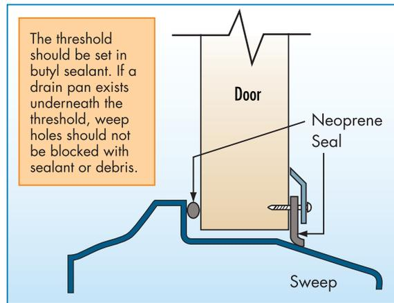
Figure 4-41: Threshold with stop and seal
