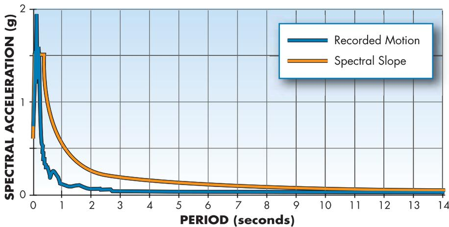
**Figure 2-36:** Response spectra for one of the orthogonal components recorded at the site of the KCH. The blue line is for the recorded motion. The orange line represents the spectral shape more commonly expected and contained in building codes.
