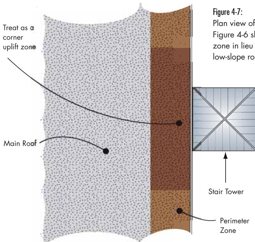
**Figure 4-7:** Plan view of a portion of the building in Figure 4-6 showing the use of a corner uplift zone in lieu of a perimeter uplift zone on the low-slope roof in the vicinity of the stair tower
