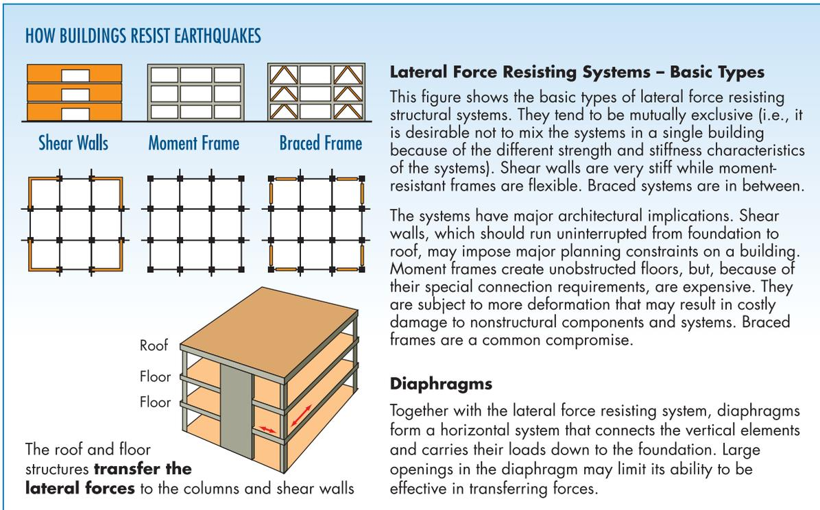
Figure 2-43: Basic types of lateral force resisting systems
