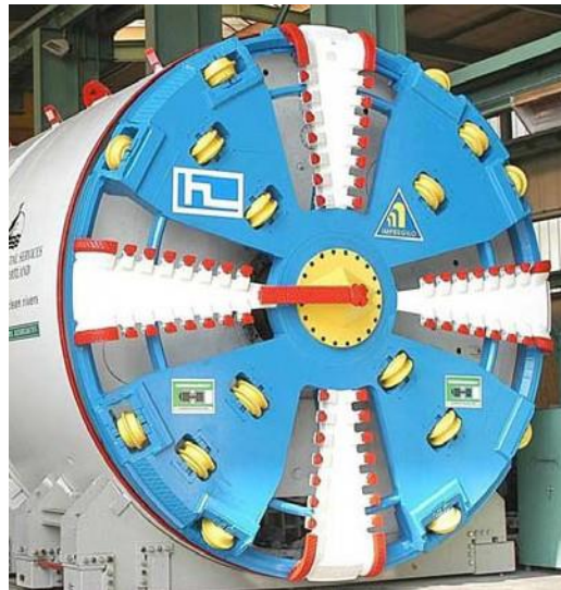
Figure 7-6 Slurry Face Tunnel Boring Machine (SFM) (courtesy of Herrenknecht).
