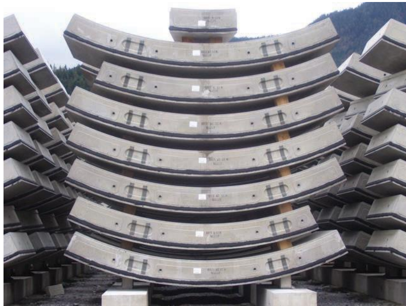
Figure 10-8 Stacked Precast Segments for One-Pass Lining
