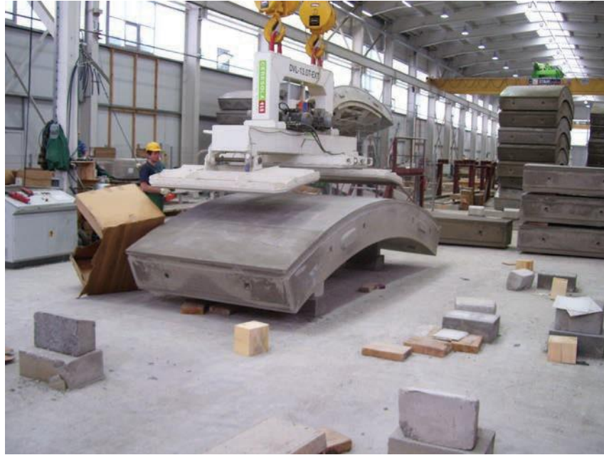
Figure 10-7 Precast Segments for One-Pass Lining, Forms Stripped
