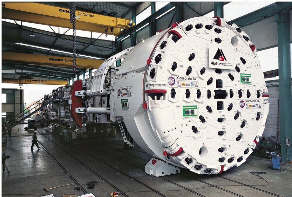
Figure D-3 Herrenknecht S-210 Gripper TBM (Herrenknecht)
