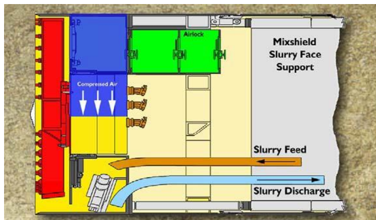
Figure 7-7 Simplified Cross-section of Slurry Face Tunnel Boring Machine (SFM) (from Herrenknecht).
