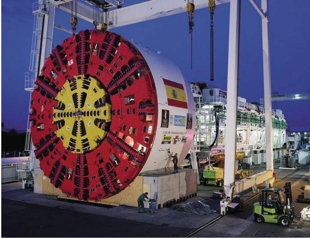
Figure D-11 The EPB Machine for the M30-By-Pass Sur Tunnel Norte project in Madrid.
