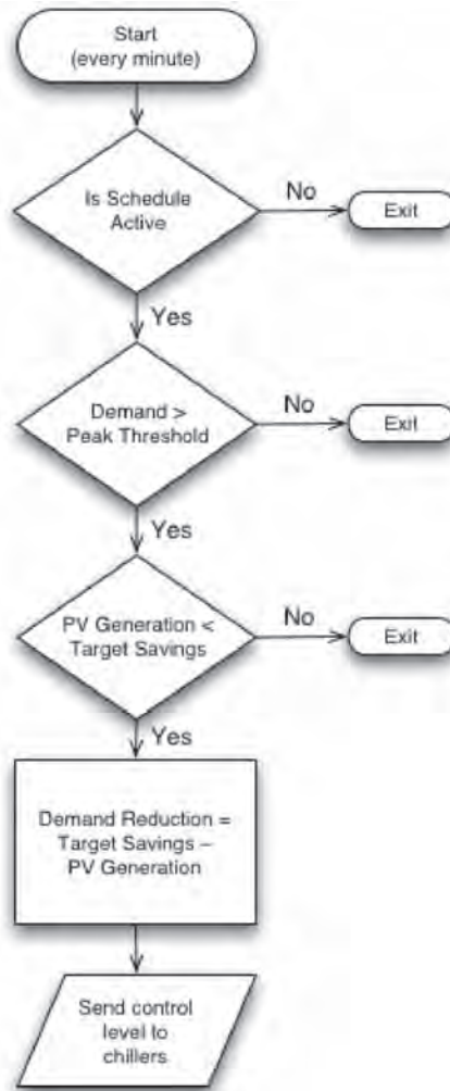
Figure 8. SLC control logic.
