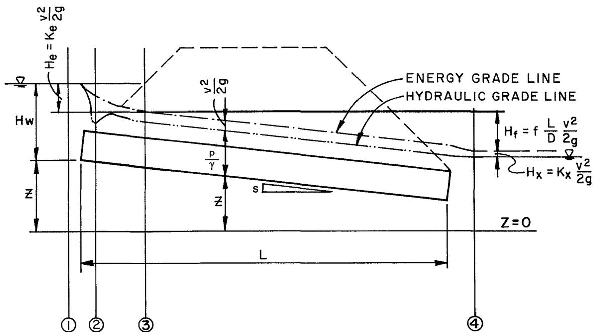
Figure CU-1—Definition of Terms for Closed Conduit Flow
