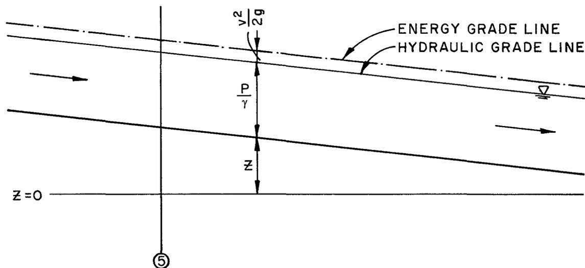
Figure CU-2—Definition of Terms for Open Channel Flow
