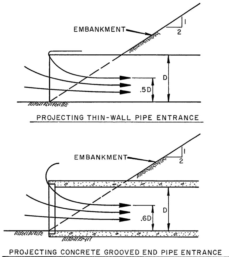
**Figure CU-11—Common Projecting Culvert Inlets**
