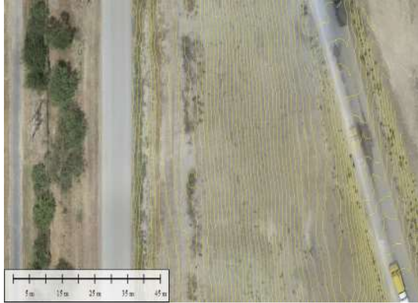
Figure 10: Topo Lines Generated by UAS
