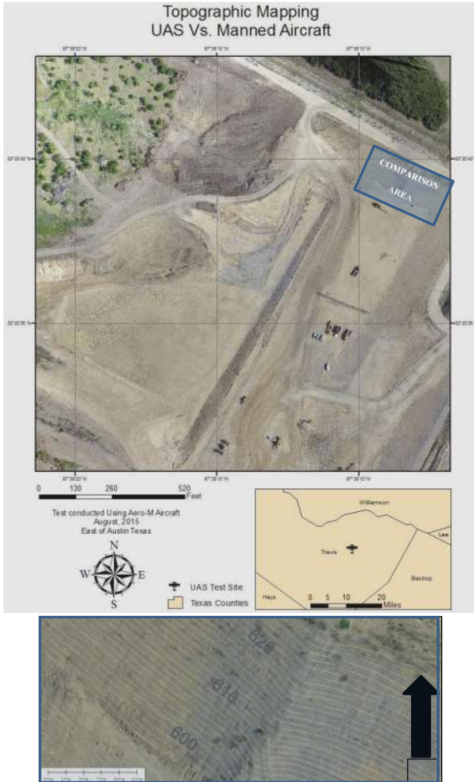
Figure 12: Top: Test Location. Bottom: Comparison of UAS and Manned aircraft Topo Lines (Lines shown in gray are from manned aircraft, lines in white are from UAS)
