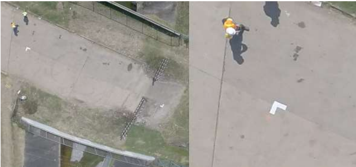
Figure 3: Example of Ground Control Points Viewed from a UAS, October 13th, 2015, Houston Texas
