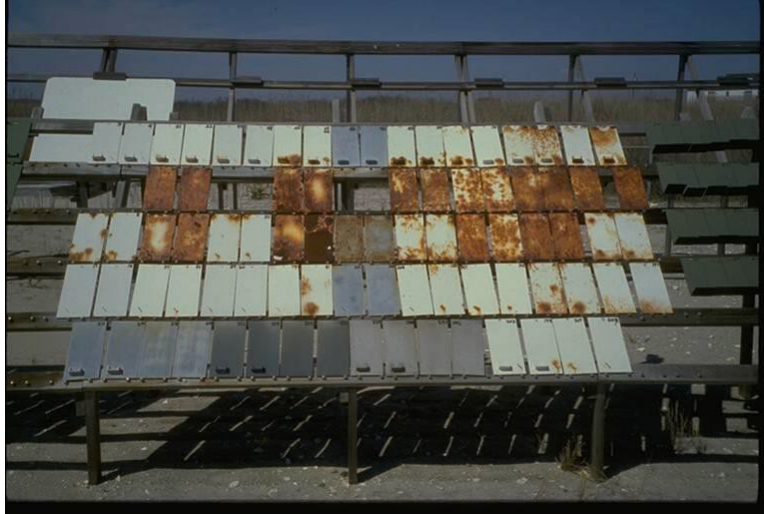
Figure 3. Photo. Testing of various generically similar paint systems shows wide variations in performance.
