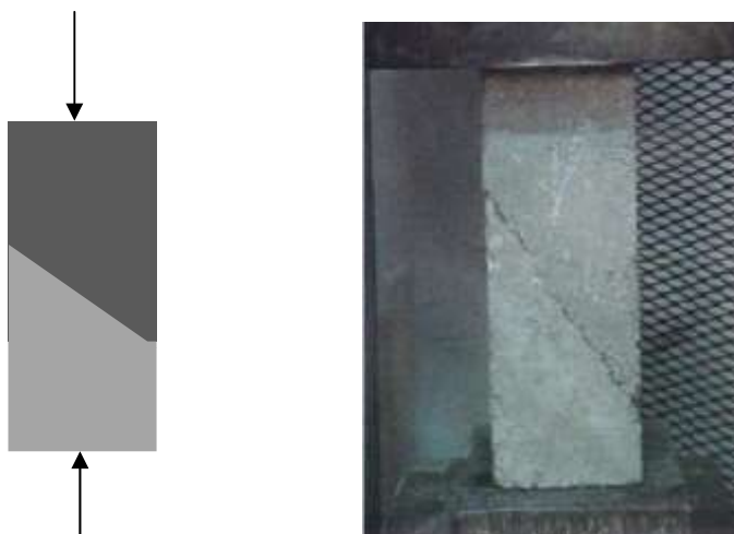
Figure 4.8. Slant shear test (Momayez et al., 2004)
