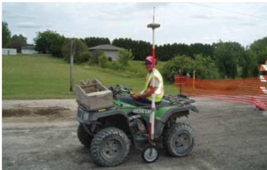
Figure 135. ATV with GPS and laser profile
