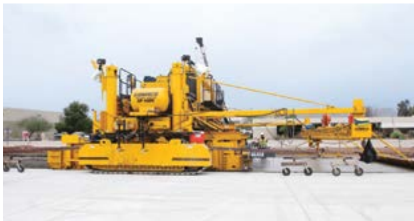
Figure 98. Controlling paving profile using a moveable stringline on the adjacent lane (source; Kevin Klein, Gomaco)
