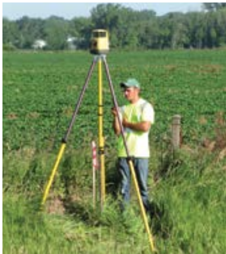
Figure 139. Rotating laser over reference points
