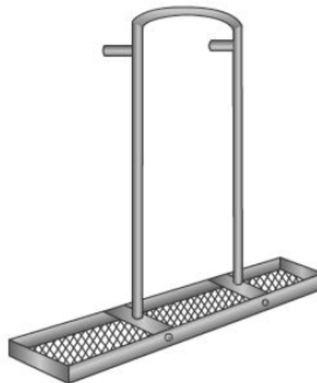
Figure 68 – Hand tamp (Jitterbug)
