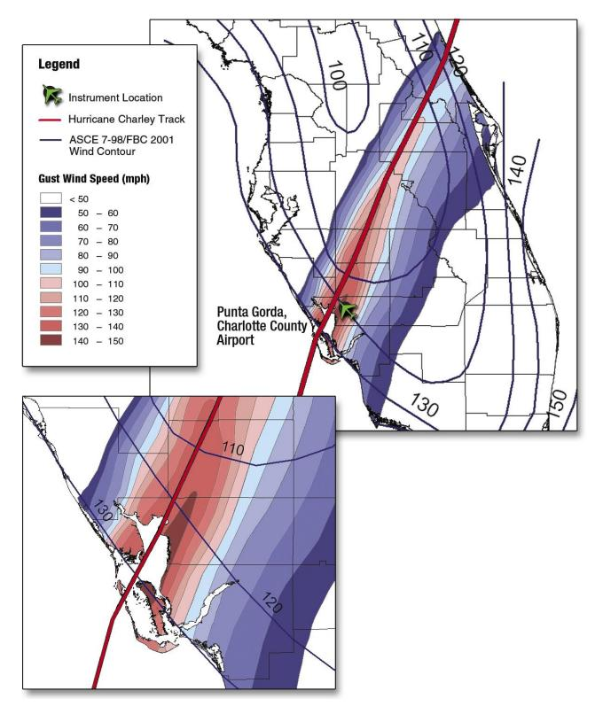
Figure 1-5. Results of the preliminary wind field analysis for Hurricane Charley based on HAZUS-MH wind methodology. The insets provide a close-up of the areas that experienced the highest winds with the design wind speed contour lines from the 2001 FBC overlaid across the wind field. (ARA)
