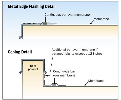
Figure 8-4. Continuous bar near the edge of edge flashing or coping. If the edge flashing or coping is blown off, the bar may prevent a catastrophic progressive failure.
