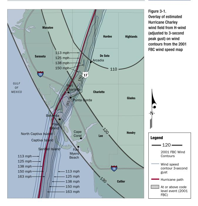
the 2001 FBC, Figure 3-1 will assist in relating damage from the wind event to the expected performance of both new and old buildings.
