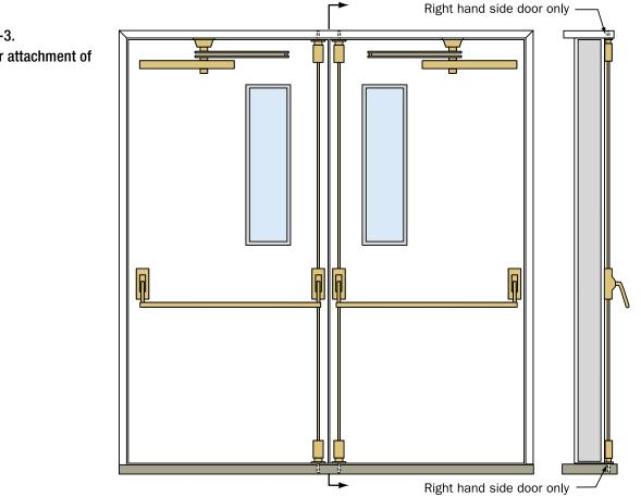
Figure 5-3. Improper attachment of doors
