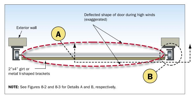
Figure 8-1. Plan view of a typical garage door
