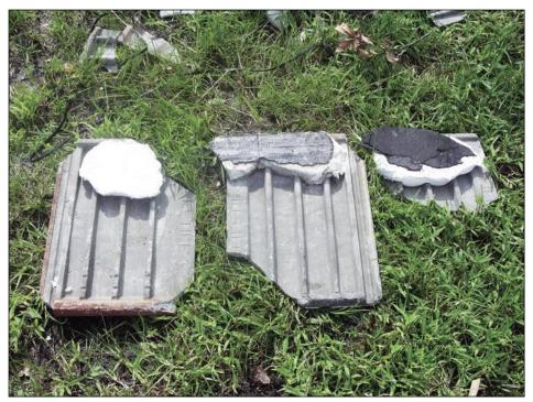
Figure 5-33. Tile debris from the roof shown in Figure 5-32 (Port Charlotte)
