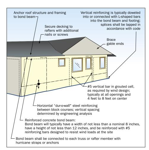
Figure 4-12. Adequately designed reinforced masonry wall system
