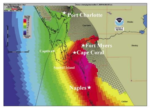
Figure 1-6. Storm surges computed using the NWS SLOSH model for Hurricane Charley, using  $R_{max} = 40$ miles
