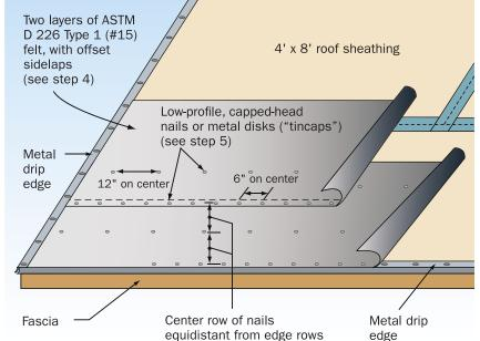
6. Fasten at approximately 6 inches on center along the laps and at approximately 12 inches on center along a row in the field of the sheet between the side laps.
