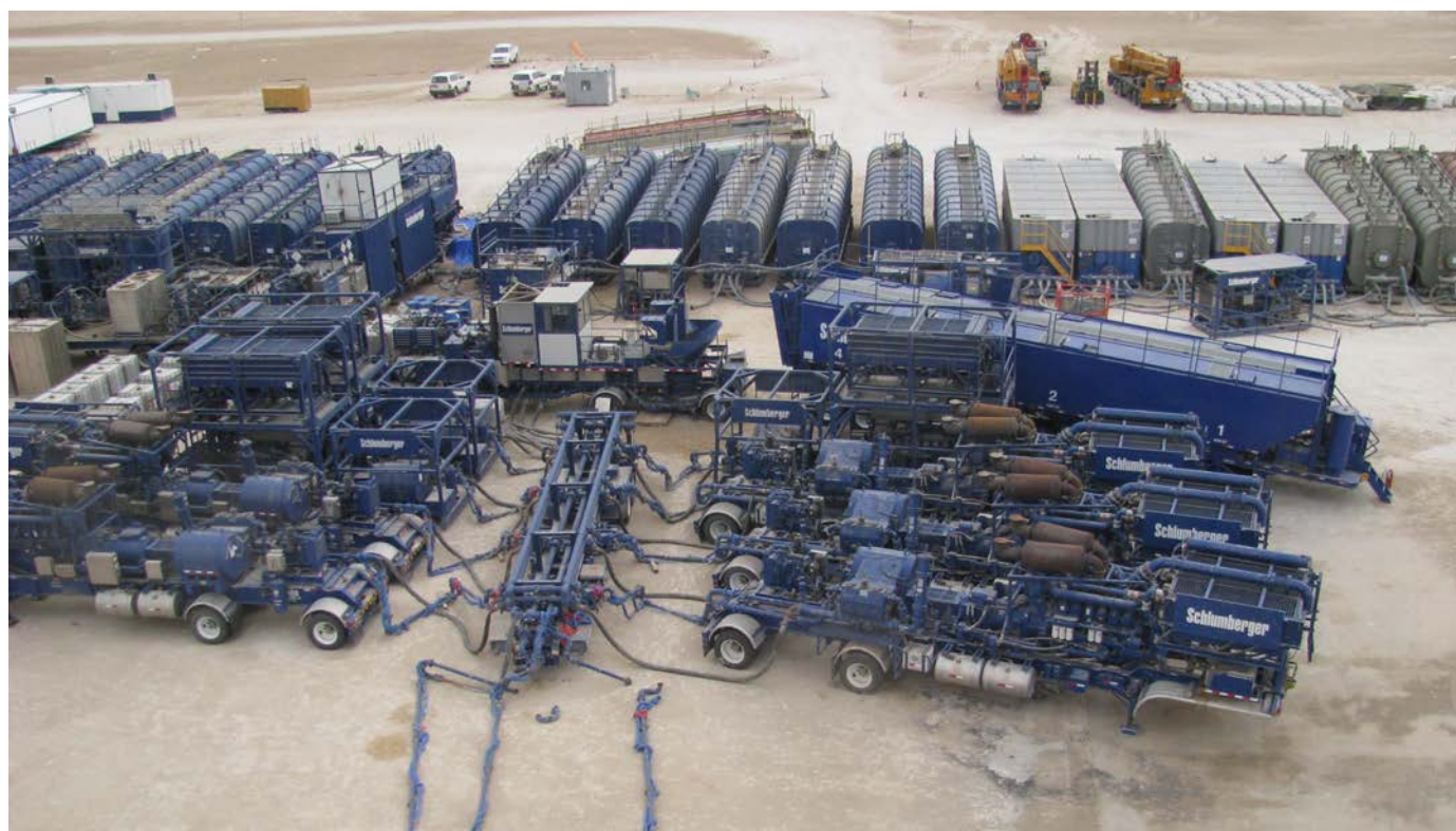
Pump trucks at BP's fracturing operations, Khazzan-Makarem field, Oman.
