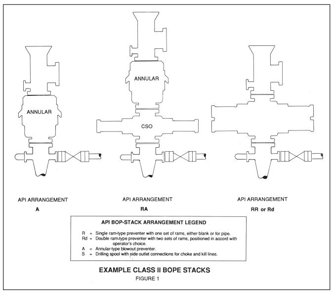
closure around the pipe in use. See paragraph 3-2a1 for additional requirements if an annular preventer is used alone (API arrangement A).
