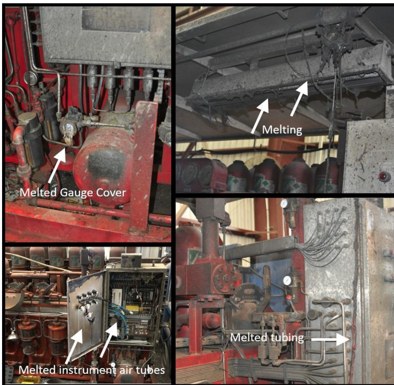
Figure A- 2. Photos of observed heat damage to Patterson Rig 219 accumulator
