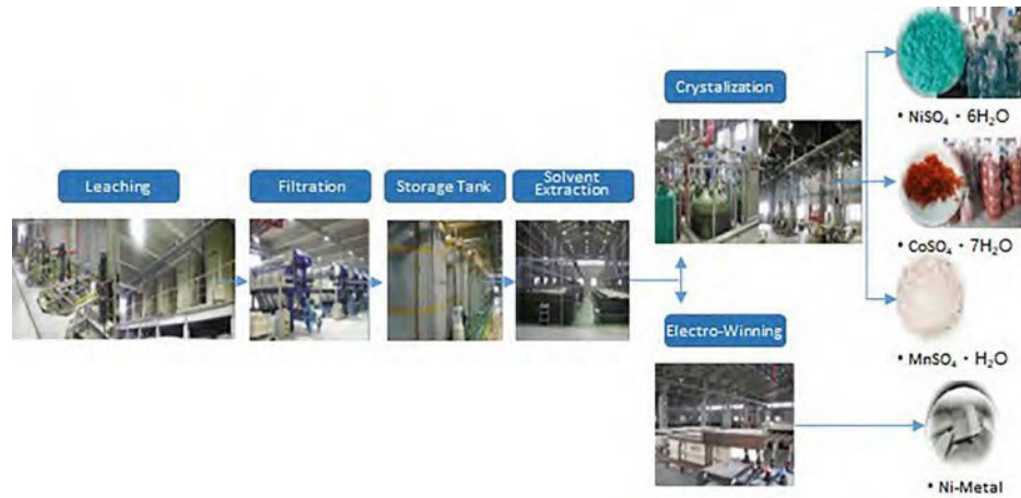
Figure 4.12: Chemical Recycling of Lithium Batteries, and the Resulting Materials
