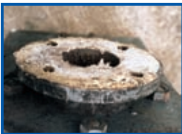
Exposed chrysotile-based compressed asbestos gasket to flange
