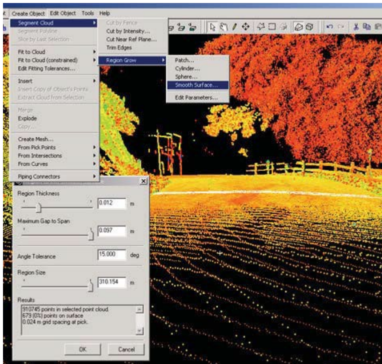
Figure 1. Screen Shot. Laser scanning software provides sophisticated algorithms for computing geometric objects and surfaces from point cloud data.
