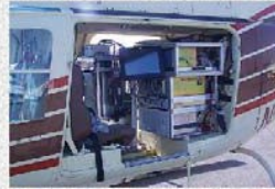
Bell 206L Helicopter. Laser and Sensor are on the left and forward. Control and data acquisition computer is on the right and aft. (Aspen Helicopter Inc.)
