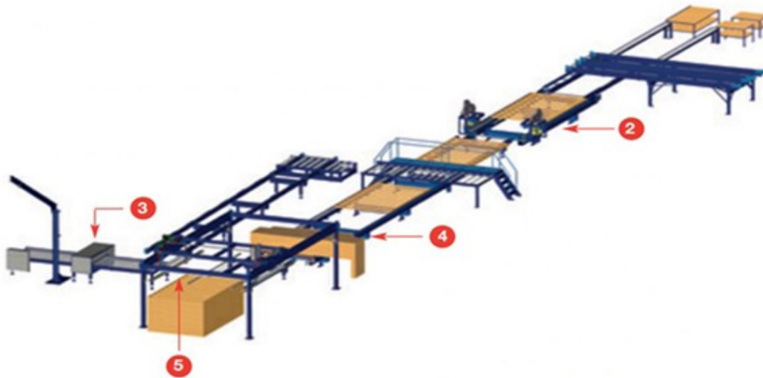
Figure 3.8 Schematic example of the MiTek panelized production line. This automated production line uses software called eFrame, which designs all the wood elements. The process starts with the component processing center, where the proper material must be loaded in the machine. After that, dimensional lumber is fed to the power framer (2) where panels move through four high production nail guns. A twin-axis sheathing saw (3) cuts the sheathing in X and Y axes simultaneously. A power squaring and sheathing station (4) attaches the sheathing to the top and bottom plates. Finally, a smart crane stacker (5) automatically stacks full levels of 16' walls and provides built-in fork pockets for easy transport of completed panels. (Source: Mitek)
