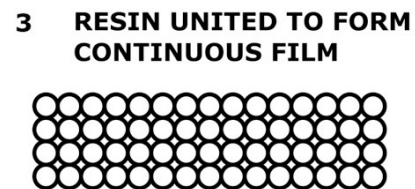
OXIDATION PROCESS EVAPORATION PROCESS Figure 2.30 Film forming with evaporation and oxidation process
