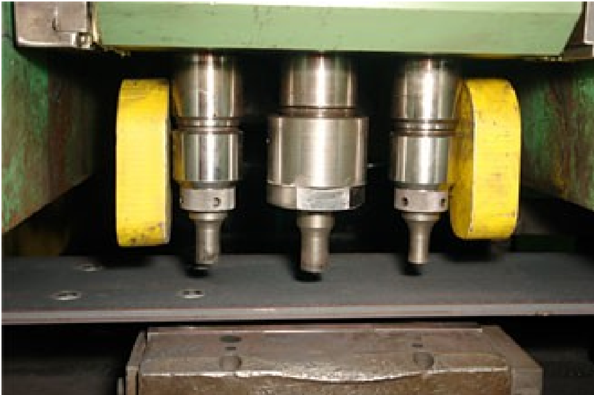
Figure 3.20 Punching of steel element is done through programming and input by the technician in charge. (Source: Butler Manufacturing)
