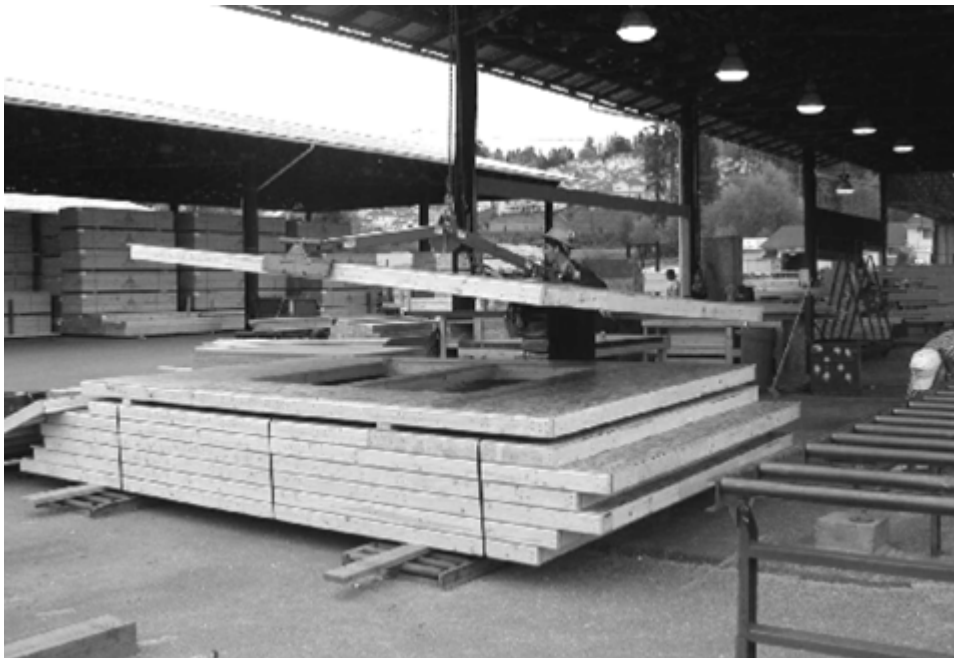
Figure 3.5 Finished panel hoisted from the production line and stacked with other panels for delivery to the jobsite. (Source: U.S. Department of Housing and Urban Development)
