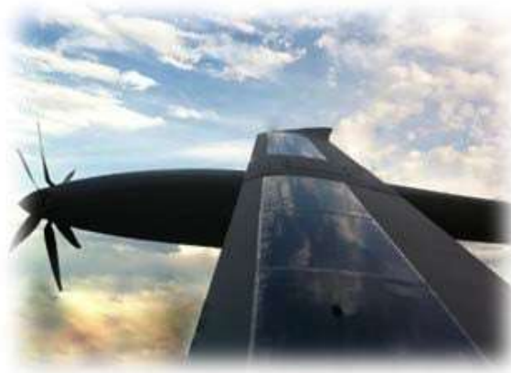
Figure 8. Solar-powered Silent Falcon sUAS 18
